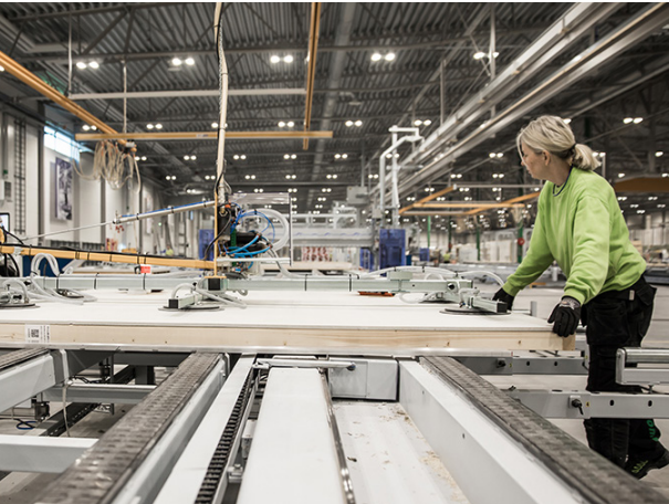
Figure 17. Photo of the assembly of the modules in the factory. (source: https://www.derome.se/bostadsutveckling/husfabriker/varo ).
