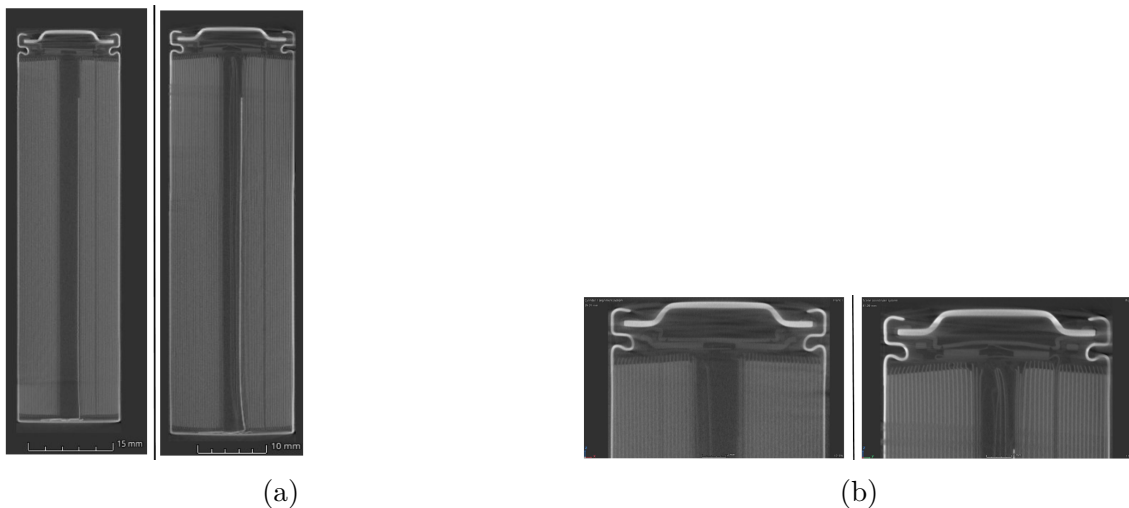
Figure 4.6: CT scans comparing BOL Cell 19 (left) and aged Cell 19 (right): (a) full cell views and (b) magnified views of the cap region.
