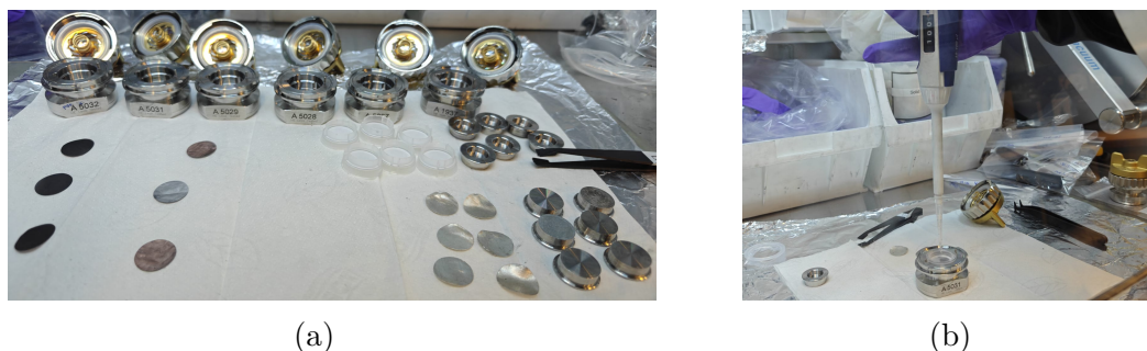
Figure 3.10: (a) All components to assemble 6 PAT-cells. (b) 100 \mu\text{L} of electrolyte was dispensed onto the separator using a pipette.
