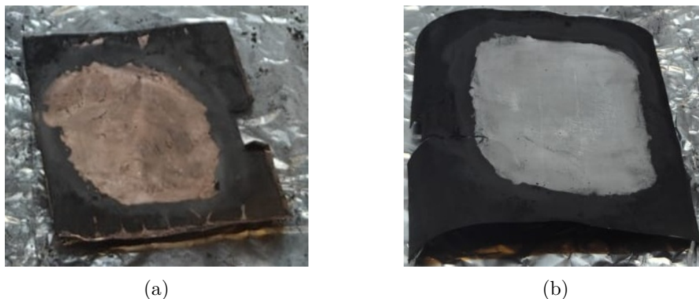
Figure 3.7: (a) Negative copper electrode after polishing. (b) Positive aluminium electrode after polishing.
