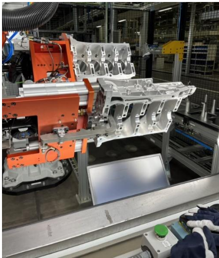
Figure 37: A picture over the quality assurance of a CB. Photo used with permission from Aurobay.
