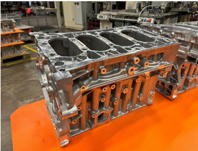
Figure 25: A cylinder block (CB) of generation 1. Photo used with permission from Aurobay.
