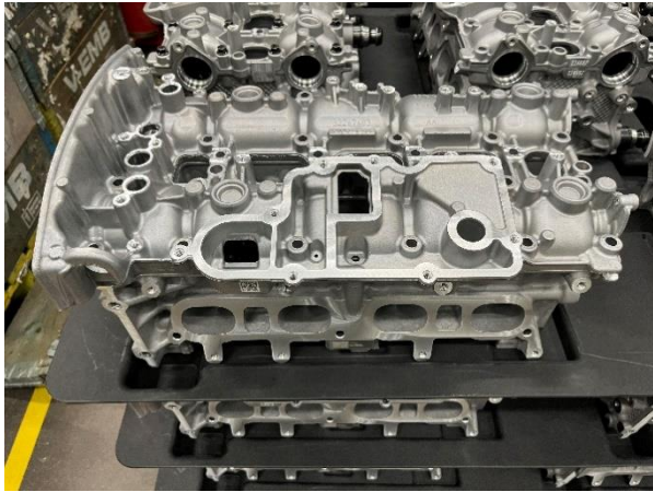
Figure 28: A cylinder head (CH) of generation 3. Photo used with permission from Aurobay.
