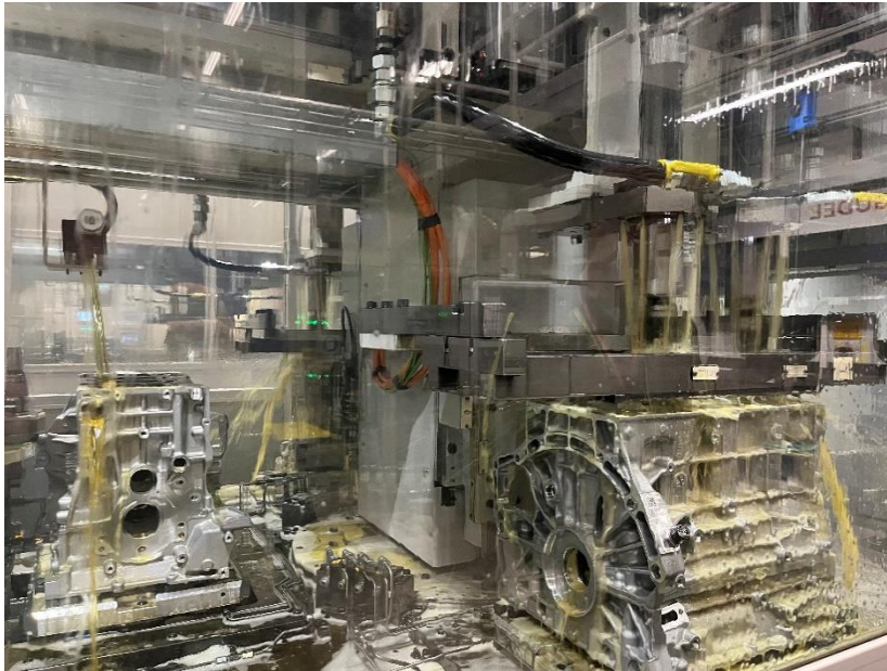
Figure 29: A picture over the process of honing a generation three-cylinder block. Photo used with permission from Aurobay.
