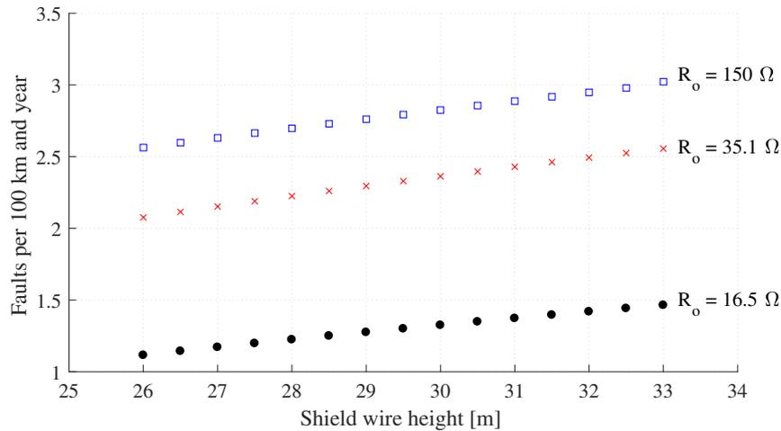
**Figure 4.3:** Back flashovers for steel tower with different tower foot resistances and different shield wire heights.
