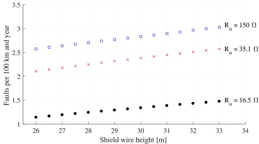
**Figure 4.6:** Back flashovers for concrete tower with different tower foot resistances and shield wire heights.
