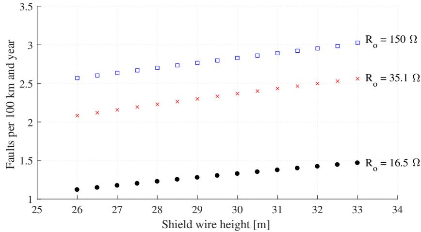
**Figure 4.1:** Total line performance of a steel tower for different shield wire heights and with different tower foot resistances.
