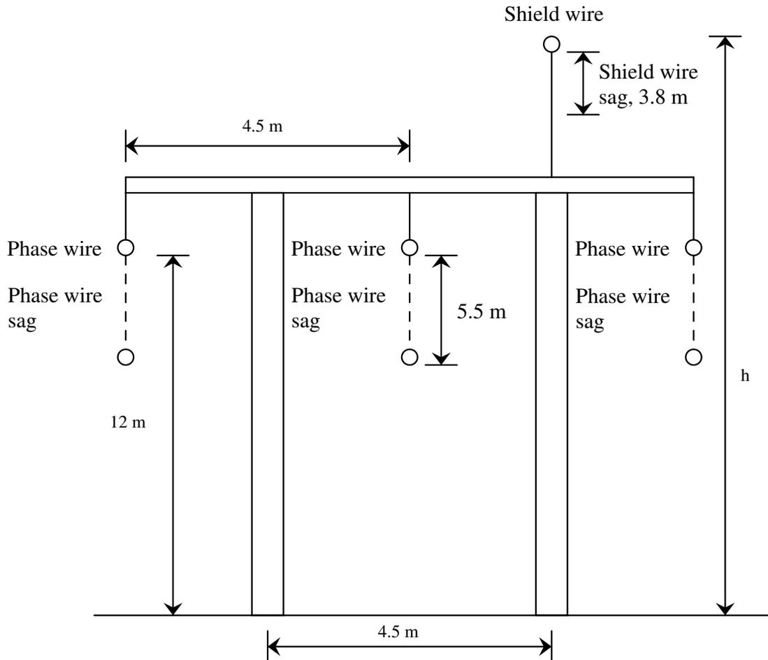
**Figure 3.3:** Wood portal tower with one shield wire.
