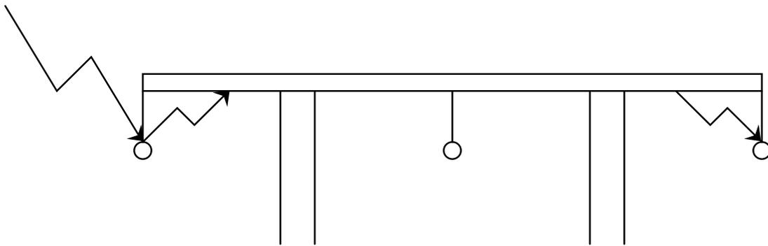
**Figure 2.4:** Two-phase short circuit due to a stroke to the outer conductor on a wood portal tower with ungrounded cross arm.
