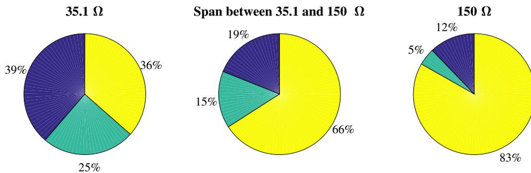
(b) Strokes to two different towers and the span between them using the second distributed model.
