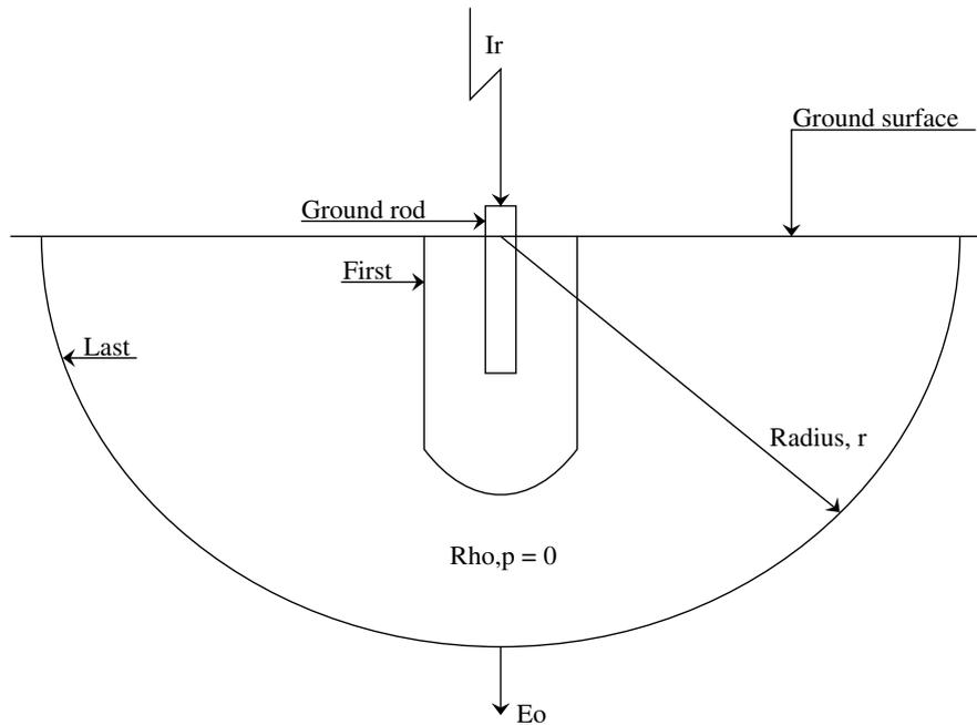
**Figure 2.8:** Ground rod acts like a hemisphere when exposed to a high current.
