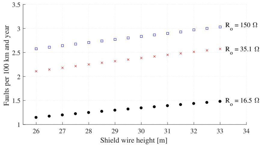
**Figure 4.4:** Total line performance for concrete tower with different tower foot resistance and different shield wire heights.
