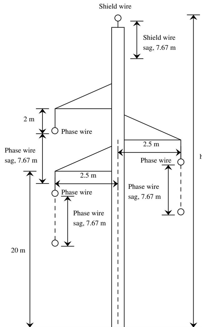
**Figure 3.6:** Steel tower with vertical phase configuration and one shield wire.
