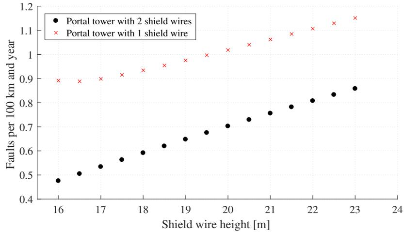
**Figure 4.7:** Total line performance for wood portal towers for different shield wire heights with one respectively two shield wires and a tower foot resistance of  $16.5\ \Omega$ .
