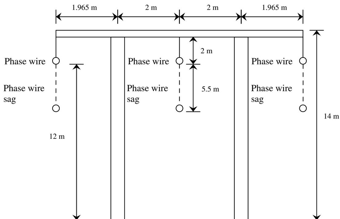
**Figure 3.2:** Wood portal tower without shield wire.
