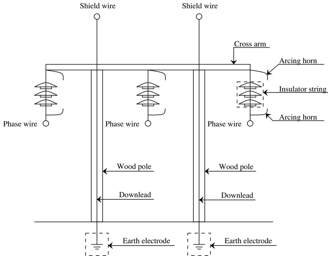
**Figure 2.2:** An example of a wood portal tower 132 kV and some of its most important parts.
