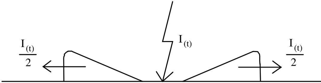
**Figure 2.3:** When the lightning stroke hits a conductor the wave is splitted up into two equal parts propagating out in each direction.
