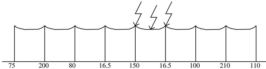
**Figure 3.10:** First distributed tower foot resistance model with lightning stroke points and tower foot resistances of poles marked.
