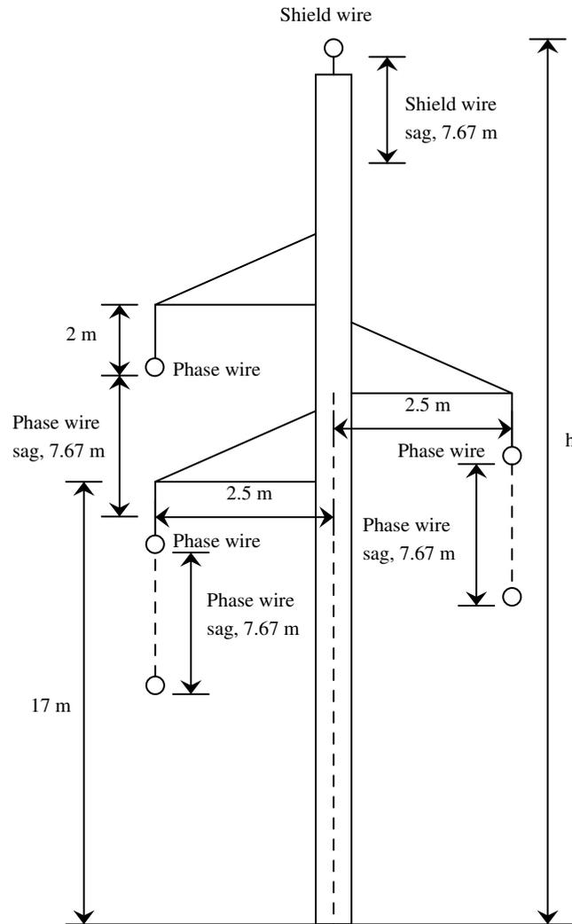
**Figure 3.7:** Concrete tower with a vertical phase displacement and one shield wire.
