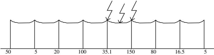
**Figure 3.11:** Second distributed tower foot resistance model with lightning stroke points and tower foot resistances of poles marked.
