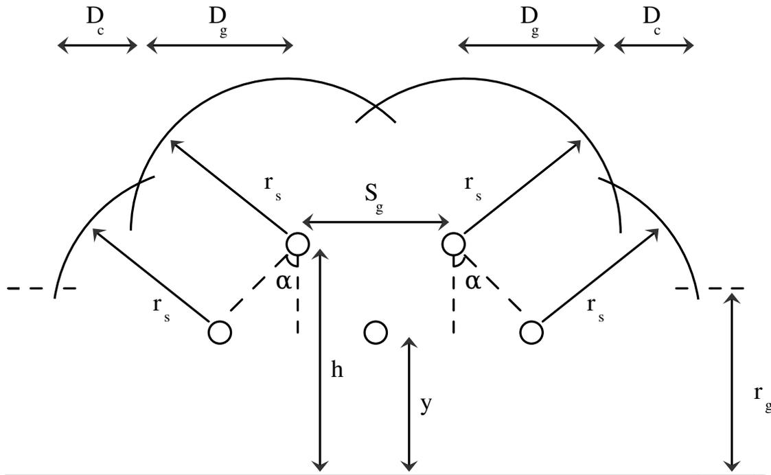
**Figure 2.6:** Electrogeometric model for a portal tower with horizontal phase configuration and two shield wires.
