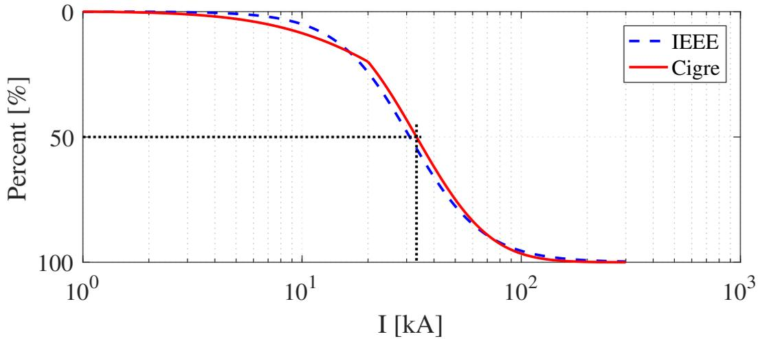
**Figure 2.1:** Probability that the lightning stroke amplitude is below a certain amplitude [1, 2].
