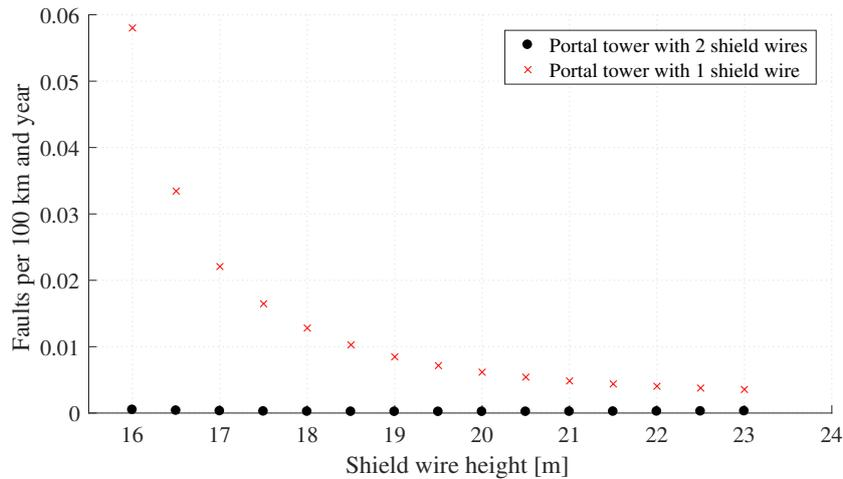
**Figure 4.8:** Amount of shielding failure flashovers as a function of shield wire height with one respectively two shield wires for wood portal tower.
