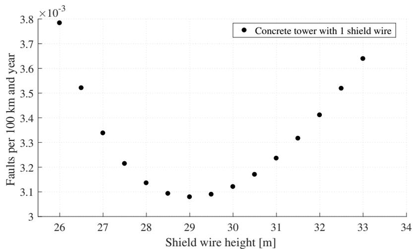
**Figure 4.5:** Amount of shielding failure flashovers as a function of shield wire height for concrete tower.
