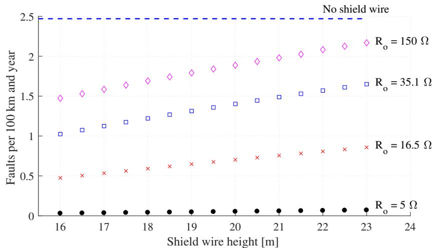
**Figure 4.11:** Total line performance for a wood portal tower without shield wire and a wood portal tower with two shield wires placed at different heights and different tower foot resistances.
