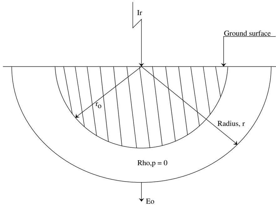
**Figure 2.9:** By assuming that the ground rod has a hemispherical shape before breakdown it is possible to describe the breakdown process mathematically.
