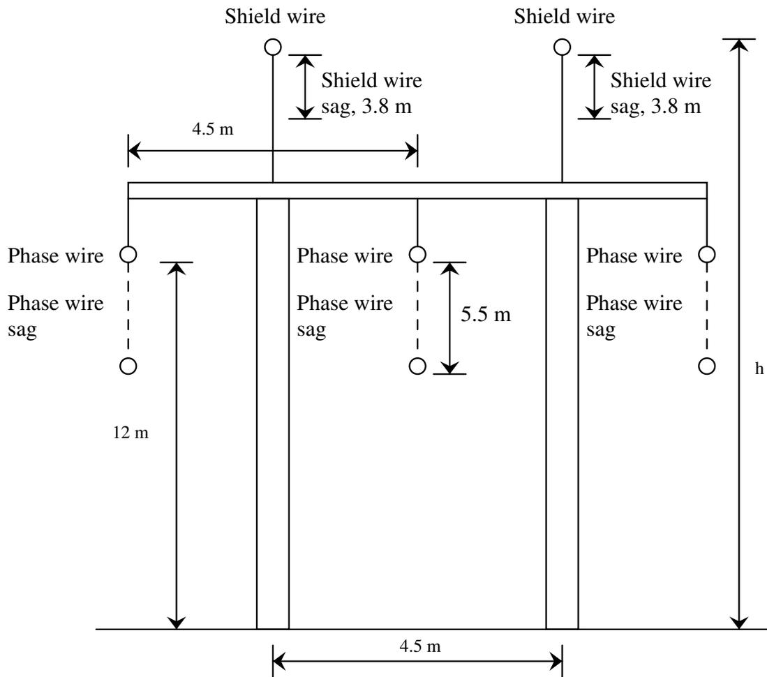
**Figure 3.5:** Wood portal tower with two shield wires.
