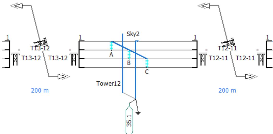
**Figure 3.9:** Portal tower with one shield wire and adjacent spans in the PSCAD model.
