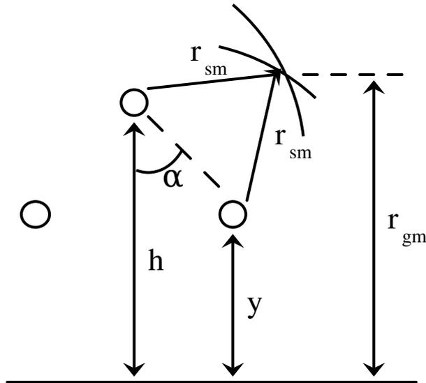
**Figure 2.7:** Electrogeometric model at maximum stroke current to phase conductor.
