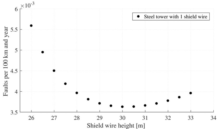
**Figure 4.2:** Amount of shielding failure flashovers as a function of the shield wire height for steel tower.
