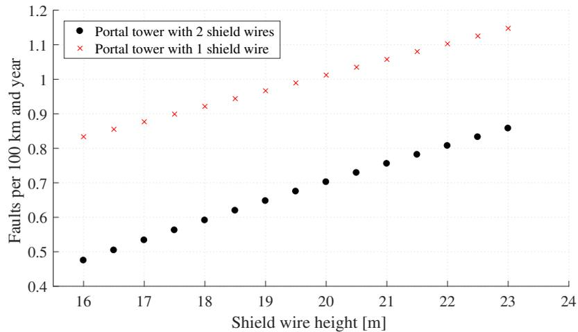
**Figure 4.9:** Back flashovers for wood portal towers with one respectively two shield wires as a function of different shield wire heights and with a tower foot resistance  $16.5 \Omega$ .
