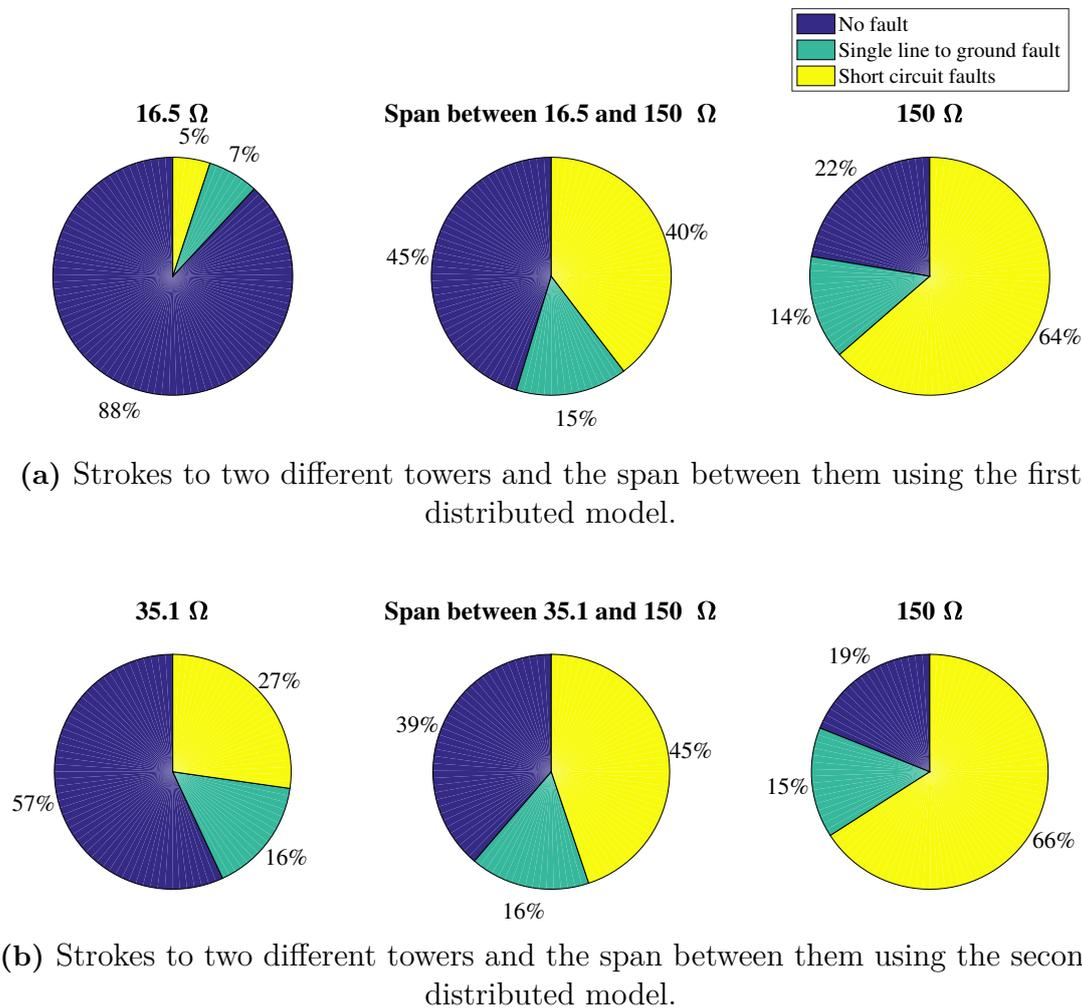
**Figure 4.17:** Fault distribution for a wood portal tower with two shield wires using the first distributed tower foot resistance model (a) and the second distributed tower foot resistance model (b). Lightning strokes hits two towers with different tower foot resistances and the span inbetween.
