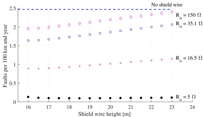
**Figure 4.10:** Total line performance for a wood portal tower without shield wire and a wood portal tower with one shield wire placed at different heights and different tower foot resistances.
