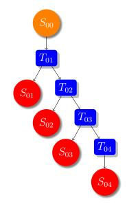
Figure 4.2: Example of a linkedlist in QML
