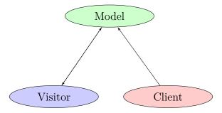
**Figure 2.3:** This figure describes the visitor pattern. The client calls *model.accept(visitor)* then the model calls *visitor.visit(model\_data)*. Then the visitor parses the top structure of the model and calls any substructures recursivly by *model\_data.substructure.accept(this)*
