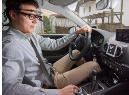
Figure 4.2: The Dikablis Glasses for Eye Tracking, one camera forward and one pointing into the eye (source: http://www.ergoneers.com/ ).
