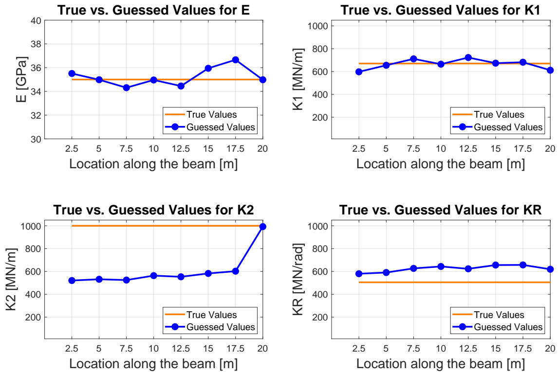
Figure 5.6: Visualisation of the variation in neural network approximations along the beam, for test Case C.
