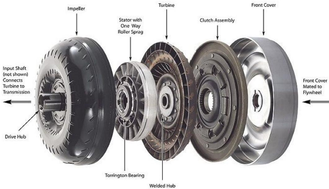
**Figure 3.3:** An exploded view of a torque converter [32].
