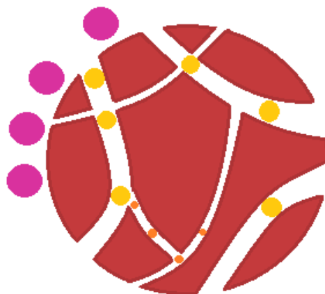
Figure 3.2: An illustration of the motion of sample and mobile phase molecules in relation to the stationary phase beads (with differently sized pores) used in SEC.
