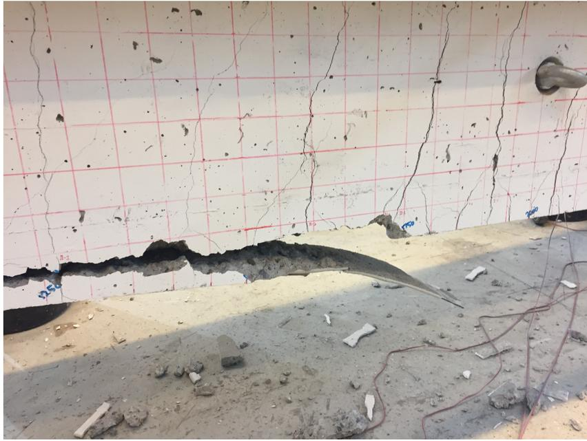
**Figure 2.4:** CFRP Failure in the Laboratory
