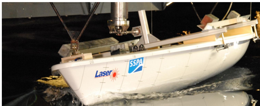
(b) Test setup during a run, loaded to an heel angle.
