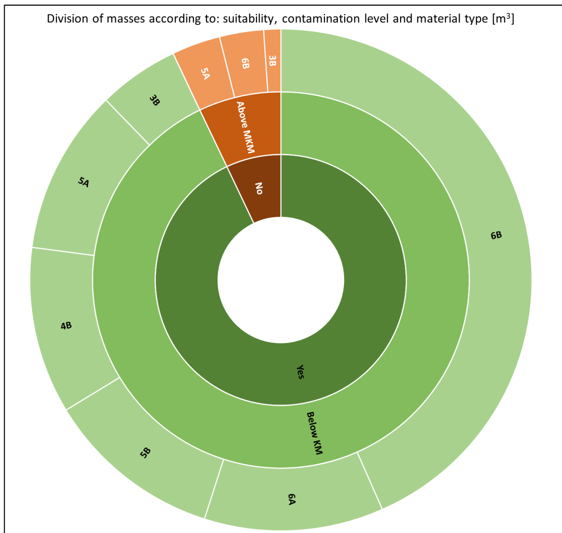
Figure 4.13 Division of masses in m 3 for project Road 41 according to suitability, contamination level and material type.
