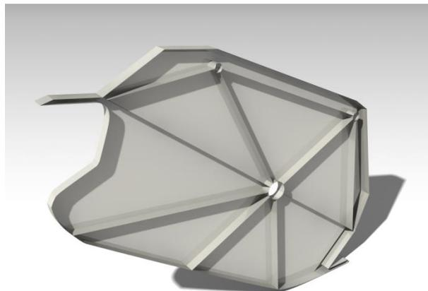
**Figure 4-1:** Sidewall panel design with circumferential fillet and outer dimensions (CTC GmbH)
