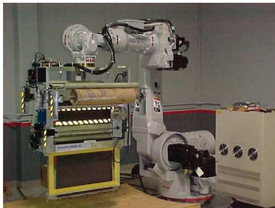
**Figure 2-11:** End effector for placing prepreg mounted on an industrial robot (Wittig, 2005)
