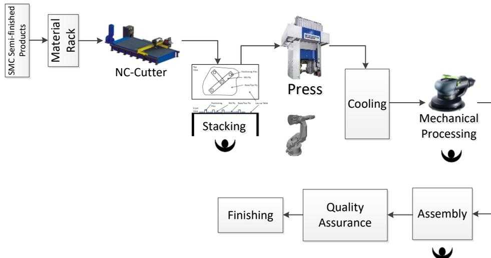
**Figure 5-9:** Conceptual line type layout for lean manufacturing approach
