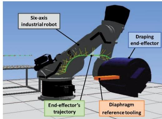
**Figure 2-12:** End effector for draping small and large dry textiles mounted at an industrial robot (Angerer, Ehinger, Hoffmann, Reif, & Reinhart, 2011)
