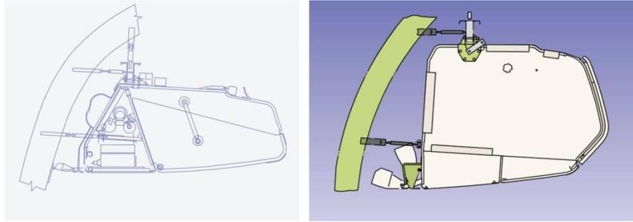
**Figure 2-8:** Illustration of a pivot bin in closed position (left) and shelf bin (right) used in Boeing aircrafts (Simmons & Worden, 2001)
