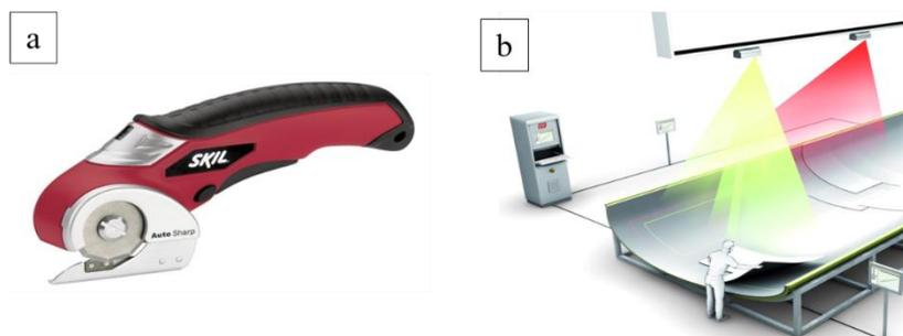
**Figure 5-5:** (a) Electric cutter and (b) laser projection system to assure correct placement of plies or preforms (focus.com, 2016) (ToolGuyd, 2016)
