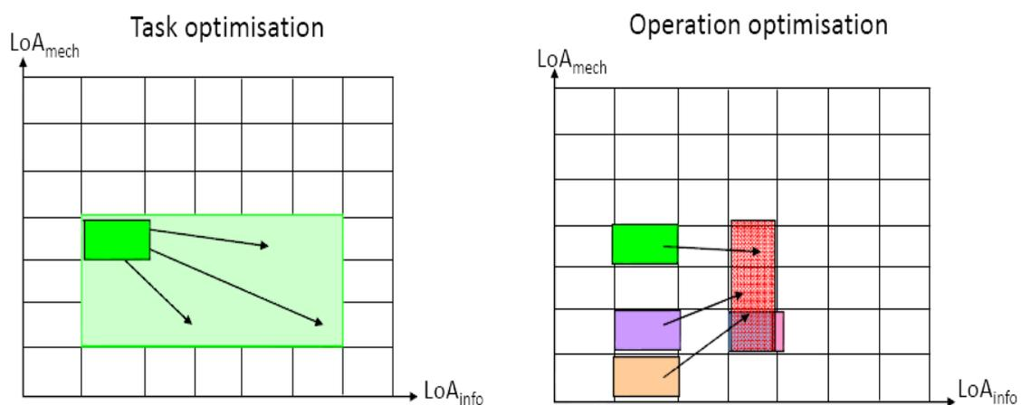
**Figure 3-2:** SoPI on task level with current level in intense green and on operation level with narrowed overlapping area (Fasth & Stahre, 2008)
