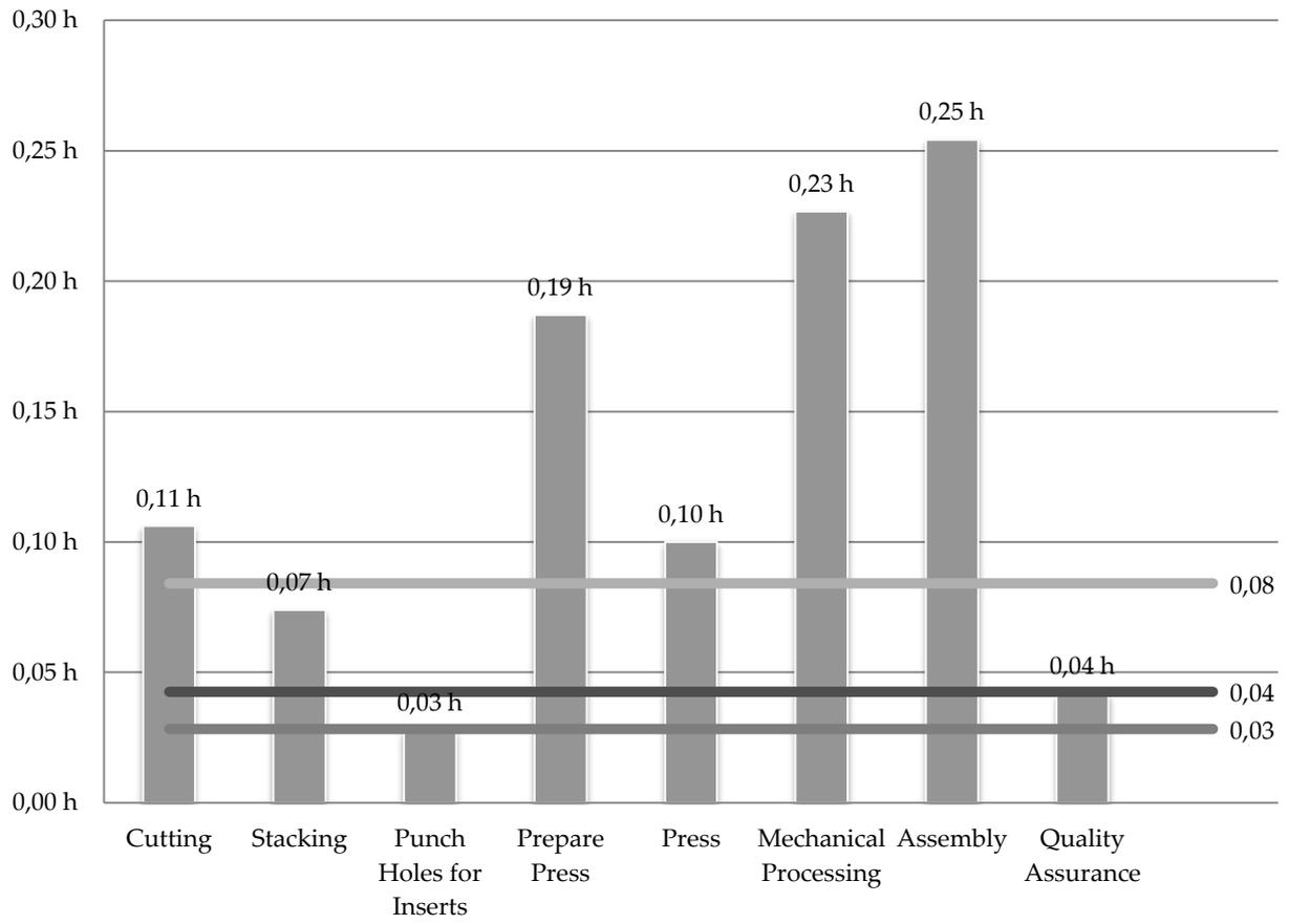
Figure 10-9: Cycle time chart of human-machine allocation approach
