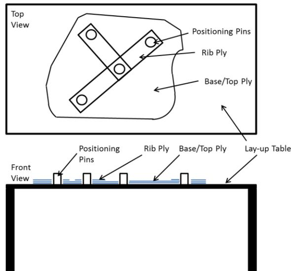
**Figure 5-7:** Template with pins to position plies and TFPs via holes cut during NC ply cutting
