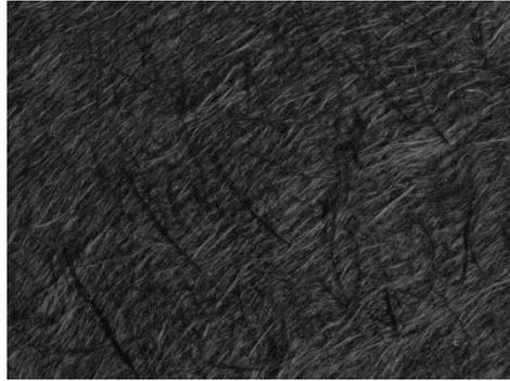
**Figure 2-5:** Needled airlaid fleece made of pyrolysed carbon fibres (Fette M. , Wulfsberg, Herrmann, Stöß, & Rademacker, 2015)
