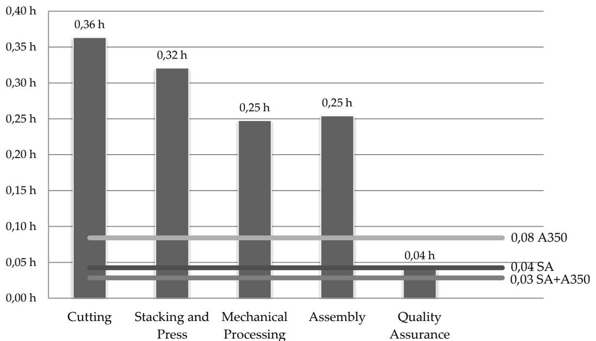
**Figure 4-10:** Plot of cycle times (bars) against the required takt times for A350, SA and SA+A350 (horizontal lines)
