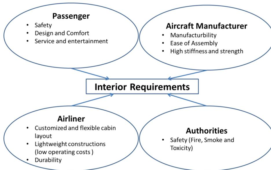
**Figure 2-7:** Aircraft interior requirements from the standpoint of different actors
