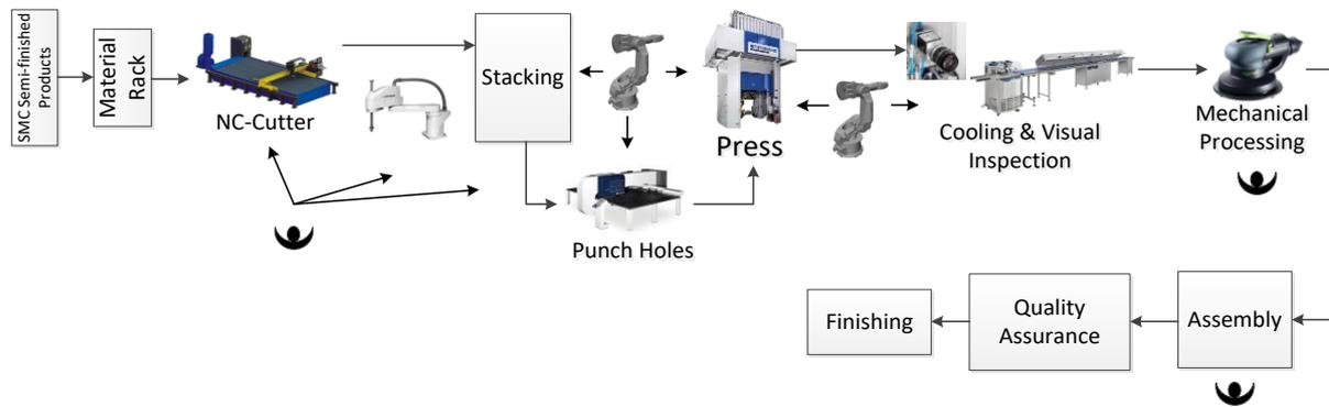
Figure 5-3: Conceptual line type layout for technocentric approach
