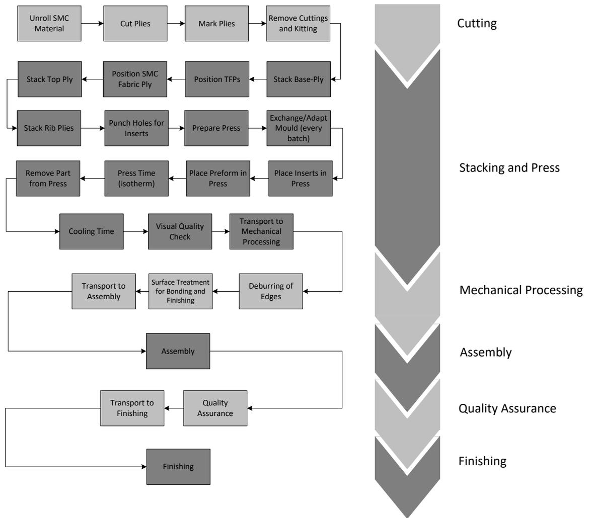
Figure 4-3: Flowchart of the sidewall production chain including assembly and paint
