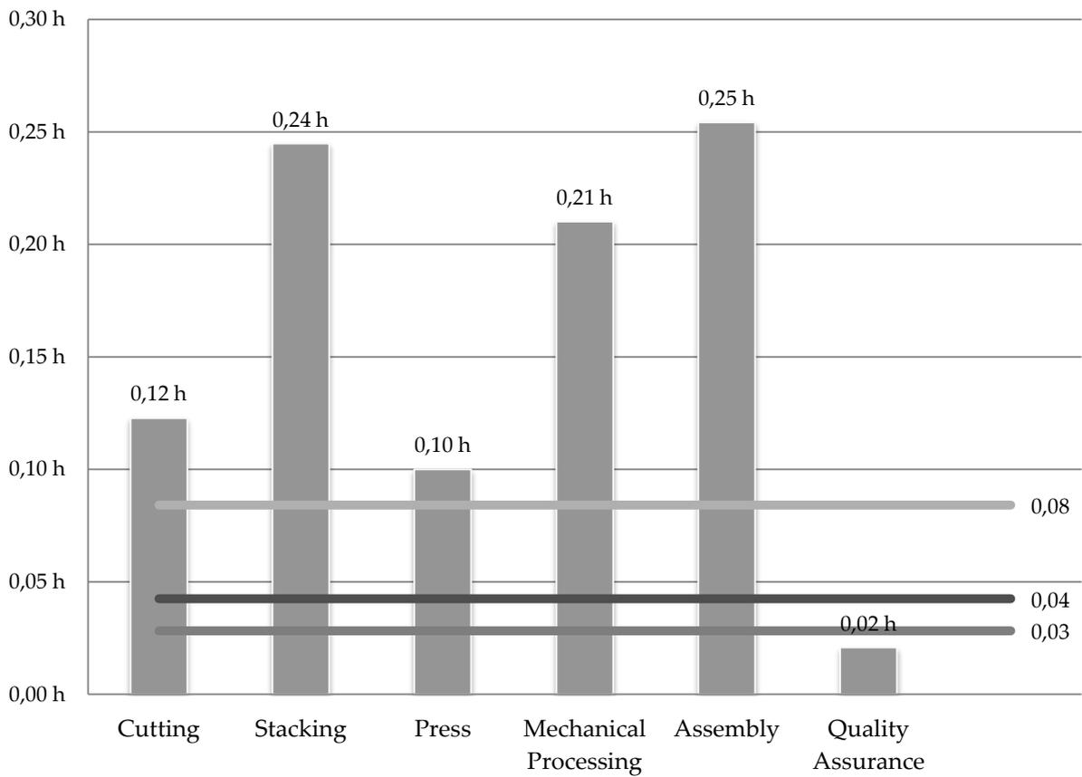
Figure 10-7: Cycle time chart of lean manufacturing approach
