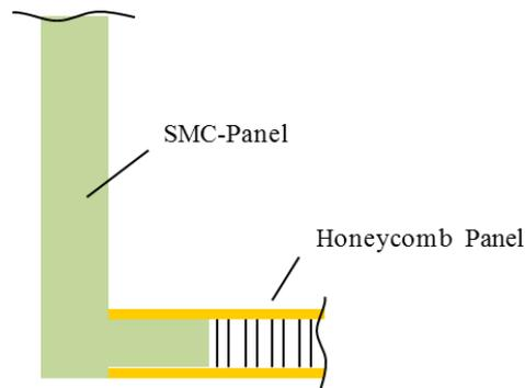
**Figure 4-2:** Schematic drawing of the sidewall panel assembly (CTC GmbH)
