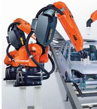
**Figure 2-10:** Articulated robots in an automotive painting line (Nof, 2009)
