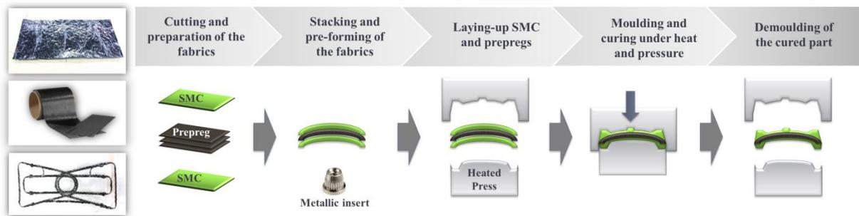
**Figure 2-3:** Compression moulding process cycle using SMC and prepreg material (Wulfsberg, et al., 2014)
