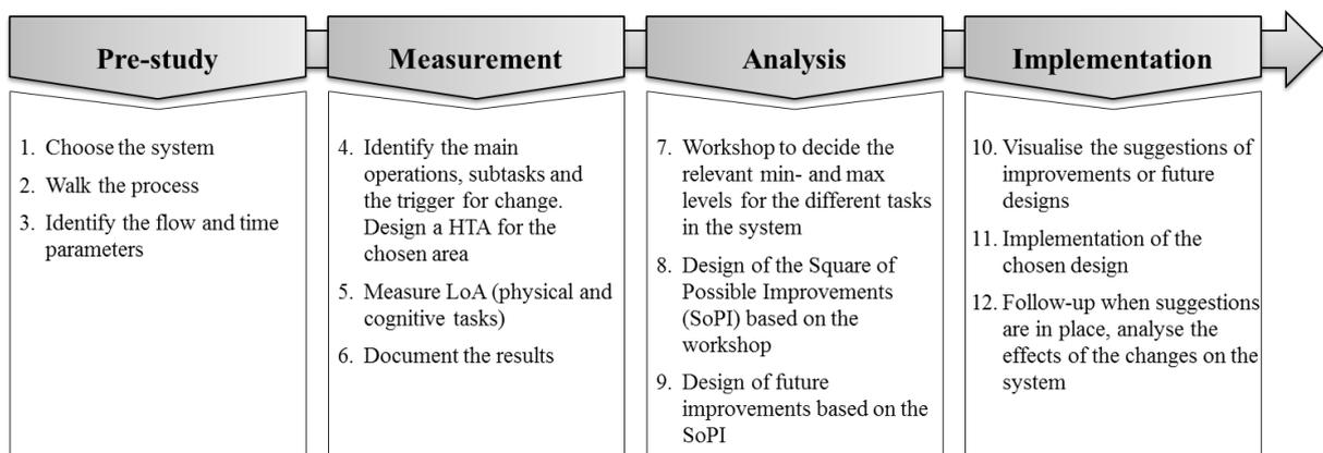
**Figure 3-1:** DYNAMO++ methodology divided in the four main phases: Pre-study, measurement, analysis and implementation (Fath, Stahre, & Dencker, 2008)
