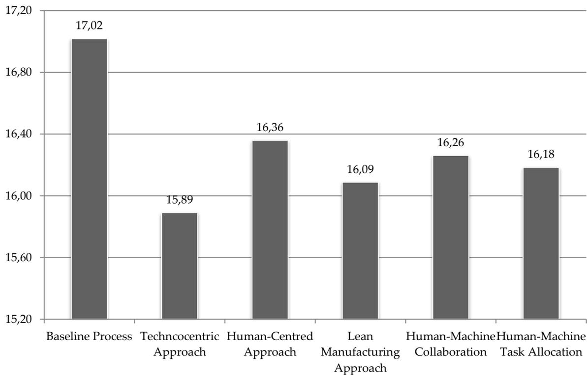
**Figure 6-3:** Production lead time according to the DES as input for the concept scoring matrix
