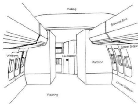
**Figure 2-6:** Aircraft interior cabin components (Committee on Fire and Smoke-Resistant Materials for Commerical Transport Aircraft, 1996)
