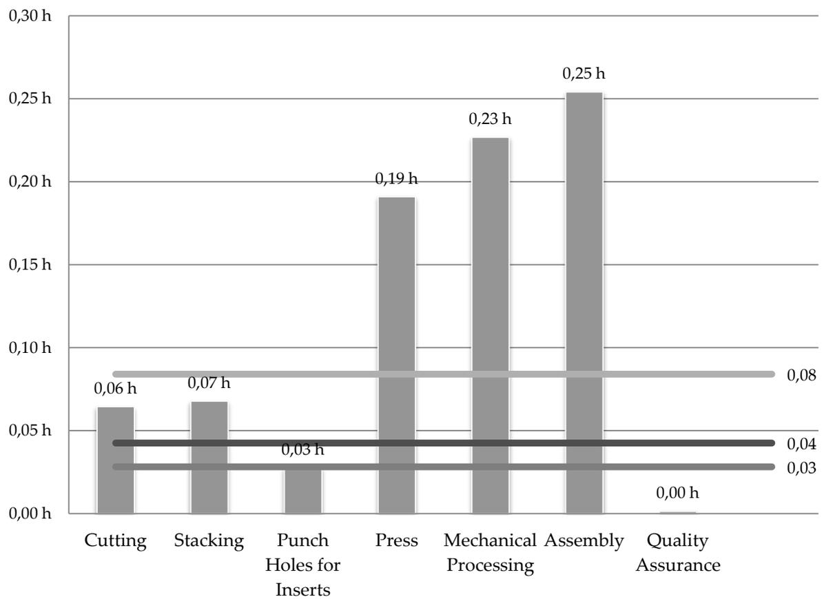
**Figure 10-5:** Cycle time chart of technocentric approach
