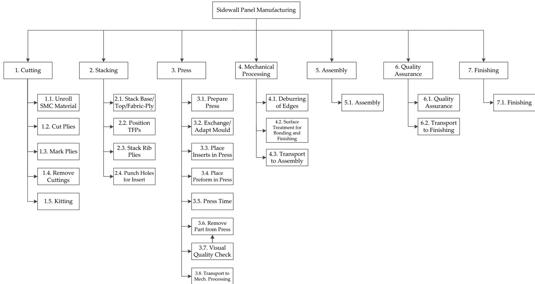
**Figure 4-13:** Hierarchical Task Analysis (HTA) of the sidewall manufacturing process
