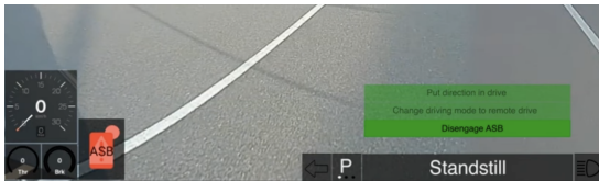
Figure 6.4: The first solution for G3 with a text-based action guide and a red ASB status element to signal that it has been triggered.
