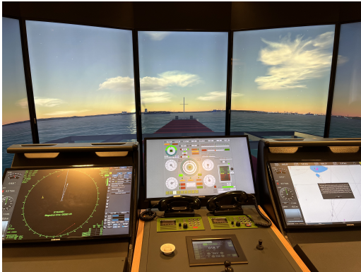
Figure 2.5: A simulator where several smaller screens are put together to form one big.
