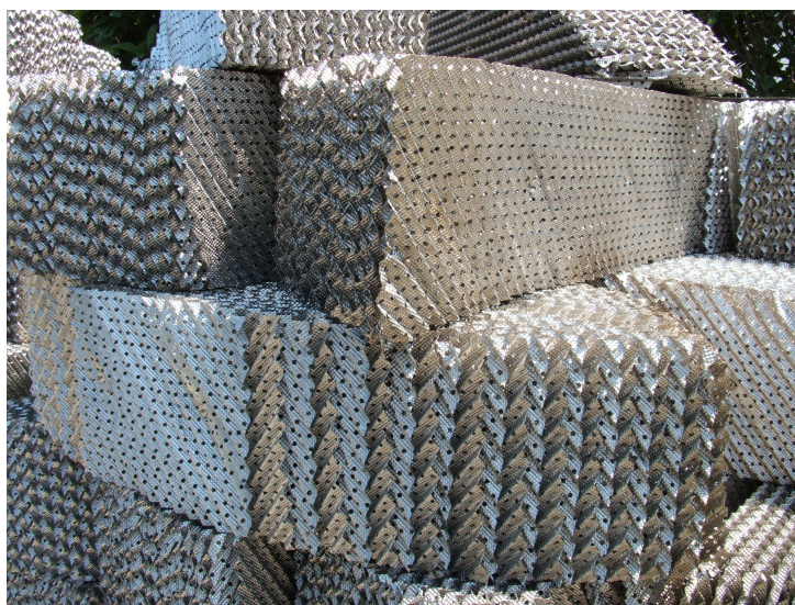
Figure 2.2: Structured packed bed material. Photograph by Luigi Chiesa. Distributed under a CC BY-SA 3.0 license.
