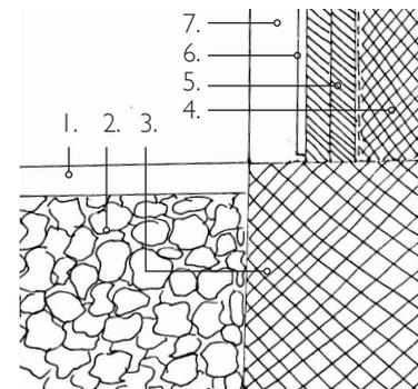
1. Hasopor (Foamglass) 2. Clay 3. Stone foundation 4. Stone base 5. Straw panels 6. Paper tiles 6. Timber structure
