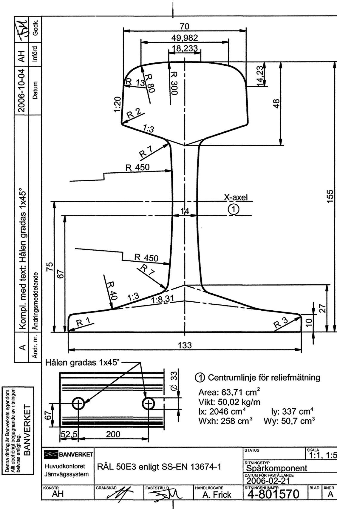
Figure 7.1: Swedish railway administration's drawing of rail profile BV50 / 50E3.
