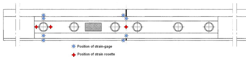
Figure 4.4: Recommended positions for strain-gauges and strain rosettes. See also figure 4.5
