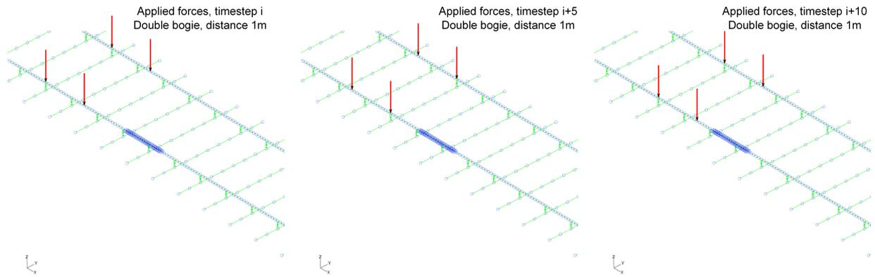
Figure 2.4: Illustration of the quasistatic approach in Abaqus for a bogie system with axle distance of 1 meter. There are five timesteps between each picture.
