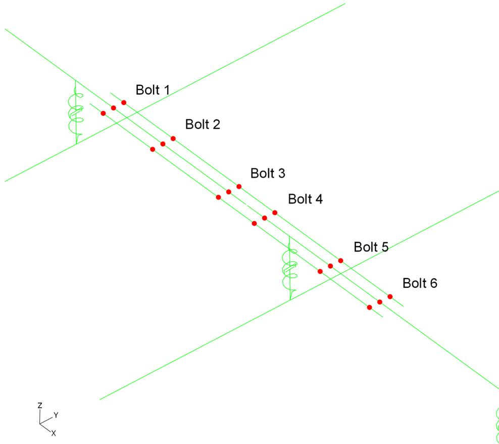
Figure 2.2: Location of bolt nodes used in the Abaqus model.
