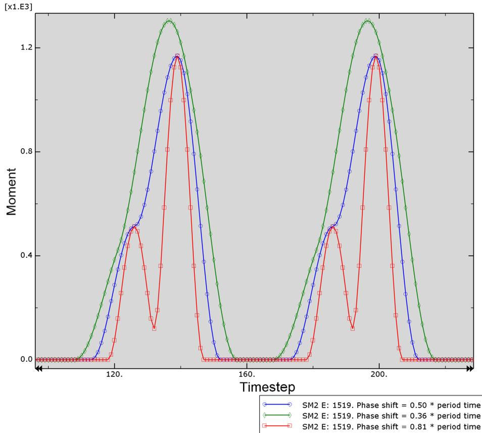
Figure 4.2: Bending moment response given the different phase shifts shown in figure 4.1. Too small phase shift (green rhombus line) gives too high bending moment response. If the phase shift is too large (red quadrat line) the bending moment response will contain additional load, which shorten the lifetime of the test specimen. Recommended phase shift is half of the period time, which in this figure is represented by the blue line with circles.
