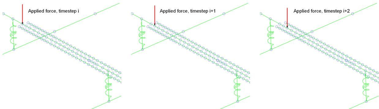
Figure 2.3: Zoomed in picture of rail 1 showing how the force is moved along the rail. An identical force with the same magnitude is applied on rail 2 (not shown in figure).
