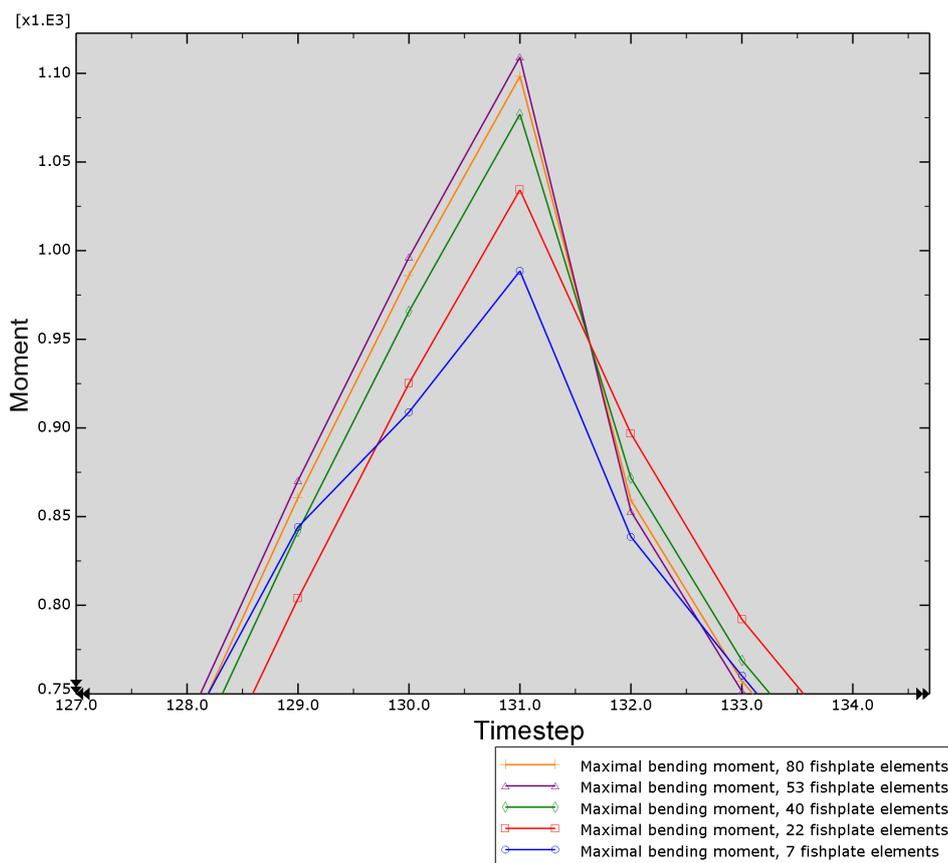
Figure 2.5: Maximum bending moment in fishplate given varying numbers of elements in the fishplate.
