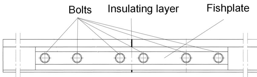
Figure 1.3: Side view of an insulated joint.
