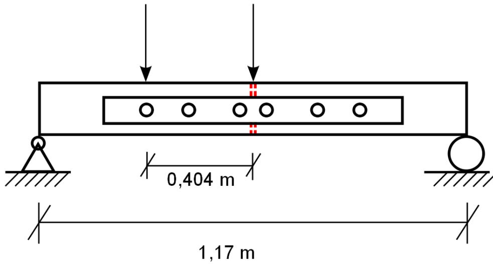
Figure 4.3: Recommended test set-up for test specimen of profile BV50.
