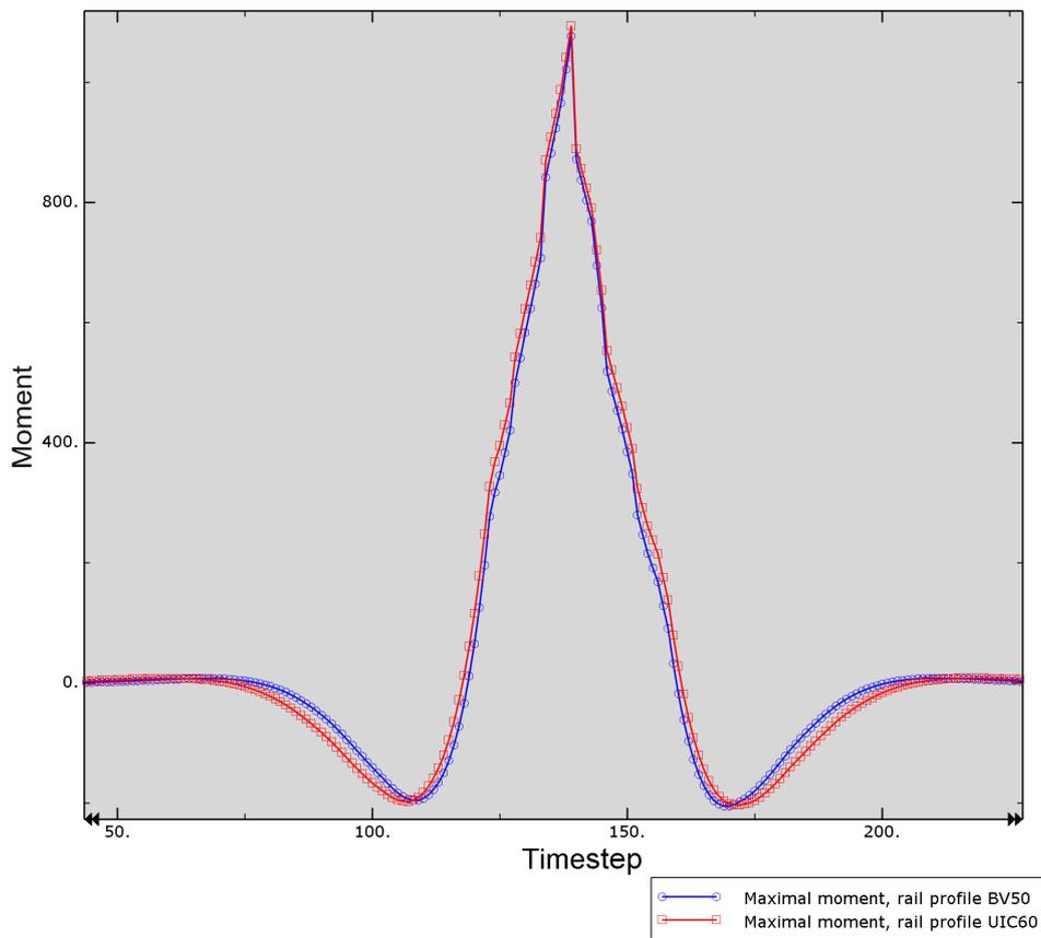
Figure 3.2: Bending moments for rail profiles UIC60 and BV50.
