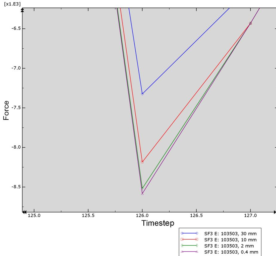
Figure 2.6: Force convergence in element closest to first bolt, applied example load 10kN.
