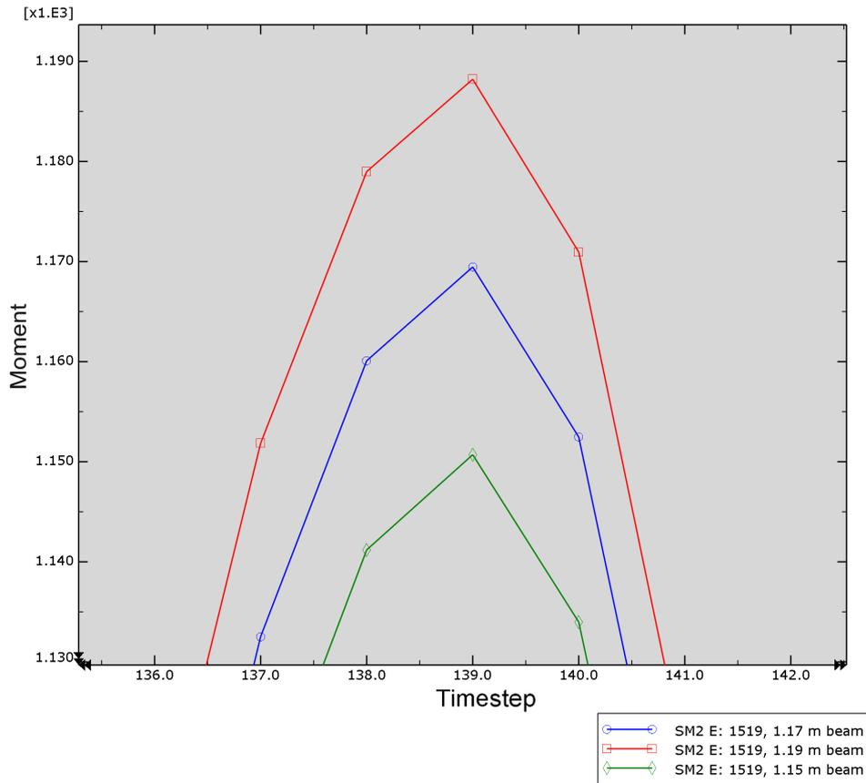
Figure 3.4: Maximum bending moment in test specimen for different lengths given an equivalent static force of  $10kN$ .
