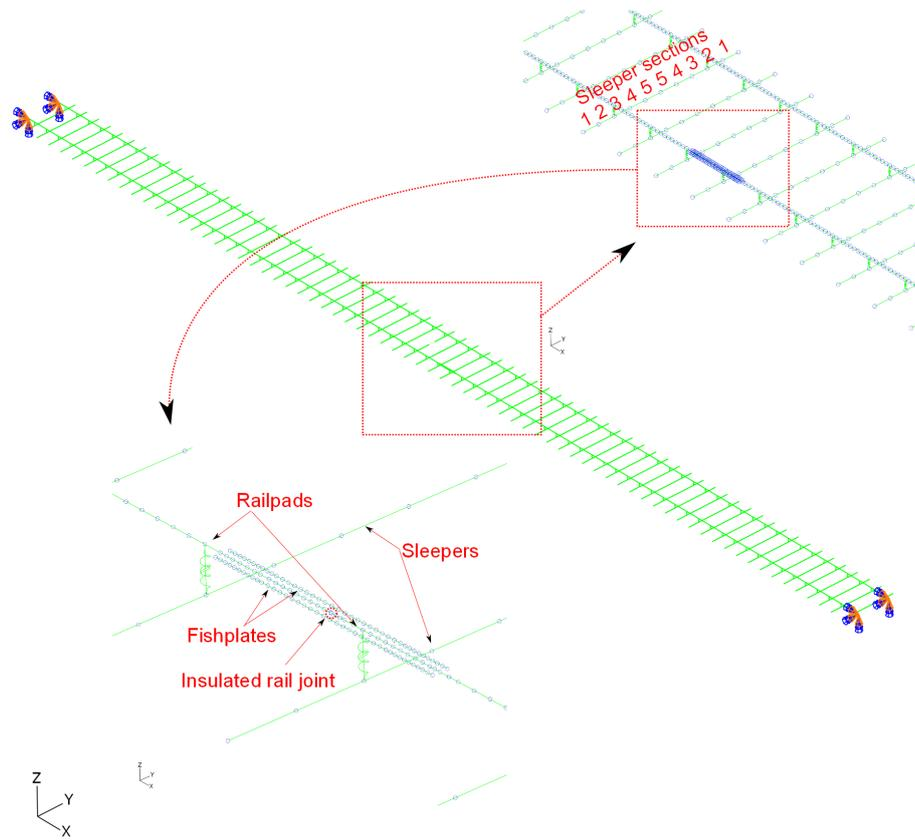
Figure 2.1: Illustration of the track model used in Abaqus simulations.
