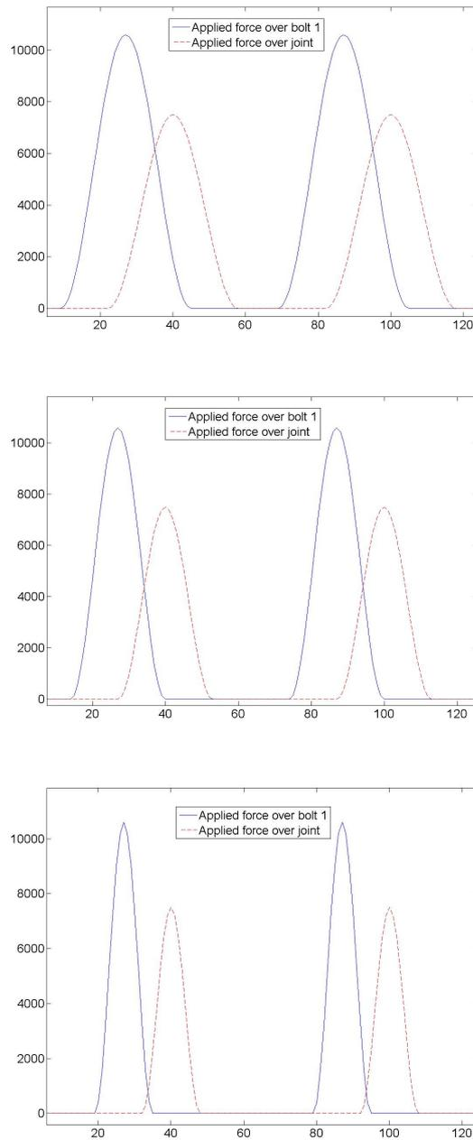
Figure 4.1: Three different phase shift profiles with phase shift of 0.36, 0.5 and 0.81 of the period time, respectively. Figure 4.2 shows the bending moment response given the different phase shifts.
