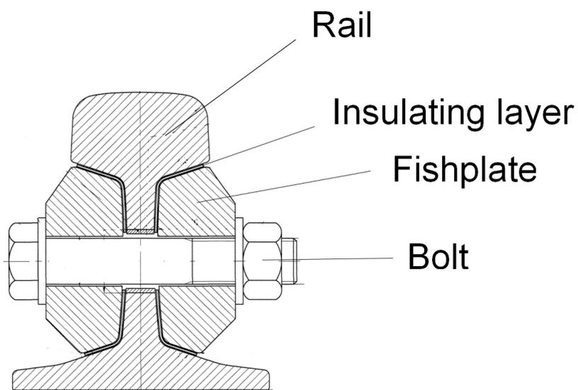
Figure 1.2: Cross-section view of an insulated joint.
