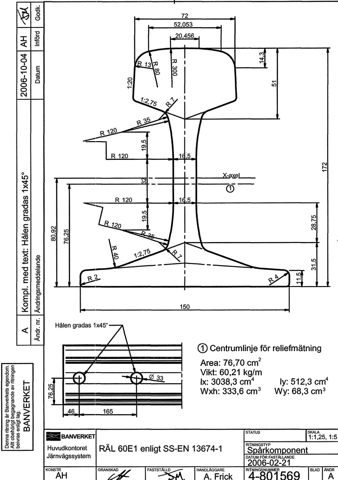
Figure 7.3: Swedish railway administration's drawing of rail profile UIC60 / 60E1.
