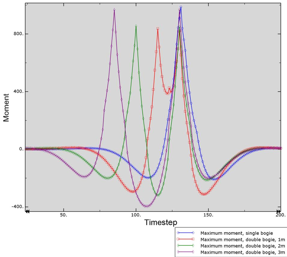
Figure 3.1: Bending moments for single and double bogie with axle distances of 1, 2 and 3 meters.
