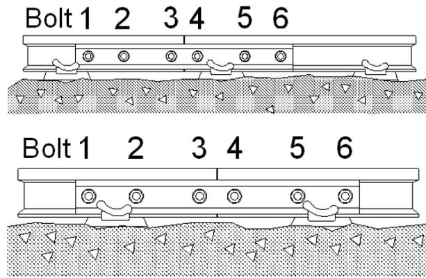
Figure 3.3: Two common positions of the insulating joint relative to nearby sleepers.
