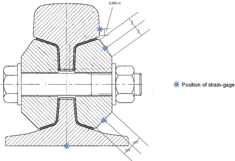
Figure 4.5: Recommended positions for strain-gauge in profile view. See also figure 4.4
