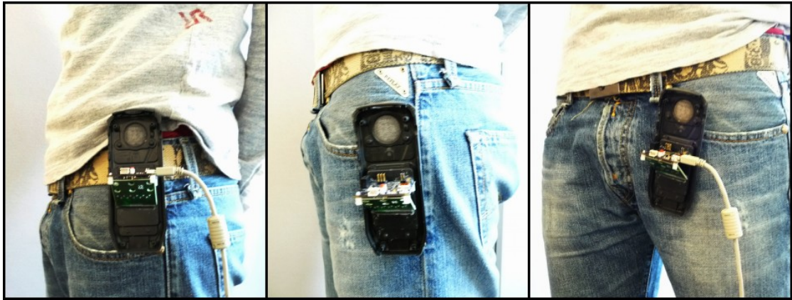
Figure 4.2: Phone positions: (left) on the waist, (center) on the left side of the left pocket, and (right) on the center of the left pocket.
