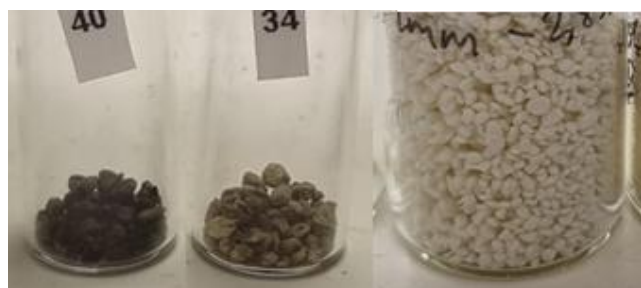
Figure 14. Granules discolored from VOC adsorption. Evenly colored granules made using point of addition A (to the left) compared to dappled granules made using point of addition B (middle). Fresh granules (to the right) for comparison.
