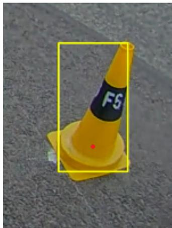
**Figure 4.1:** *A photo showing the bounding box placed by the YOLO-microservice on a distorted image. Removing the distortion of the image distorts the bounding box. The red dot marks the approximate centre of the bottom of the cone, which is the point of interest.*
