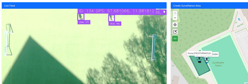
Figure 4.11: Screenshot of the video feed covering the area selected in the interactive map and detecting two persons.
