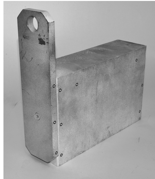
Figure 5.9: Specimen with applied surface pattern and markers.
