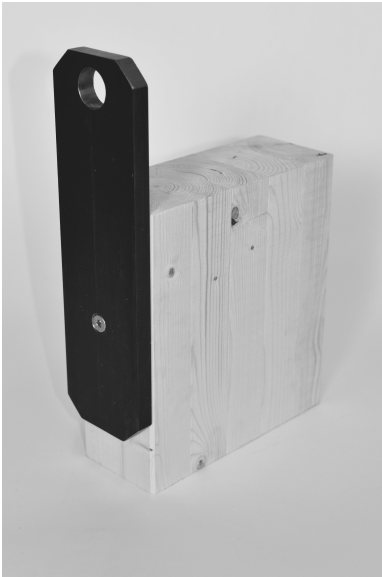
Figure 5.8: Specimen with mounted steel plate with 90° screw angle.
