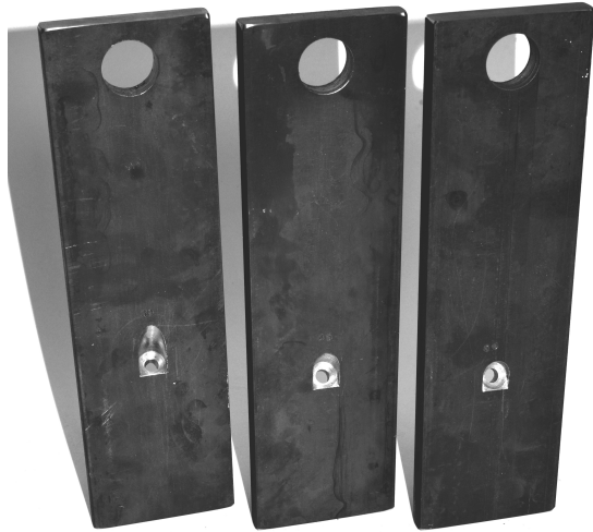
Figure 5.2: Steel plates machined for varying screw inclinations.
