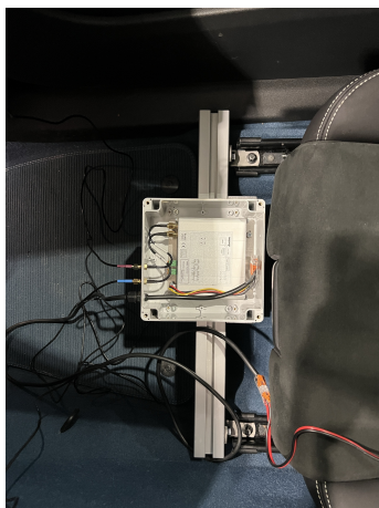
Figure 4.3: IMU in car
