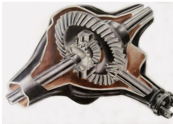
Figure 2.18: Ring-and-pinion differential structure overview[7]
