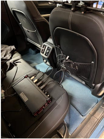
Figure 4.5: Sound Card Setup
