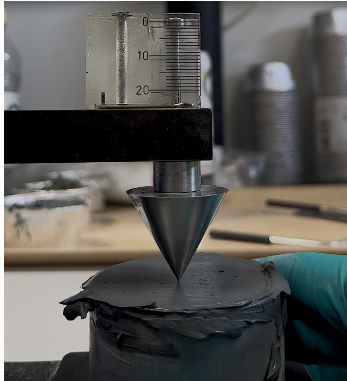
Figure 2.1: Fall cone test set up for reading of a remoulded sample equipped with a manual ruler with 1 mm measurement resolution
