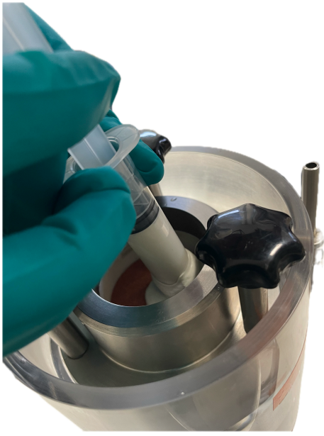
Figure 4.8: 95% slurry placed into cell using a syringe
