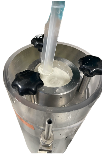
Figure 4.9: 55% paste packed into cell
