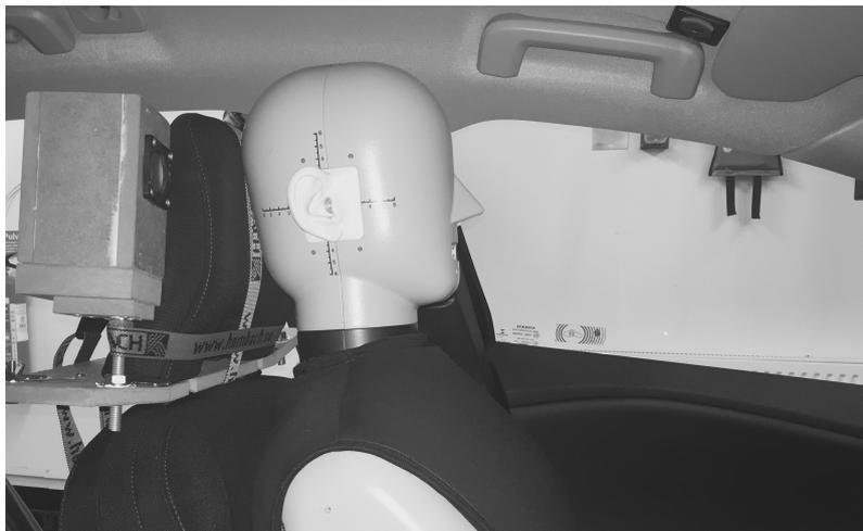
**Figure 3.5:** Picture from setup *Test rig 2*. The right front driver is seen mounted in the ceiling in the top right corner of the picture.
