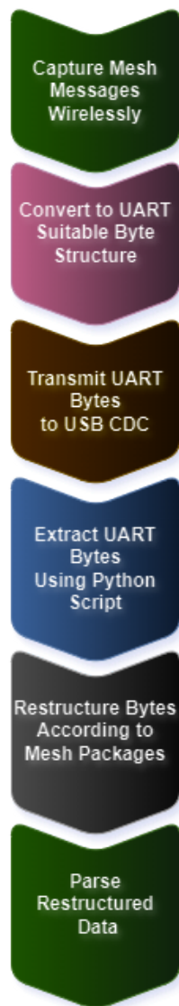
Figure 3.2: Capture and Processing of Mesh packet Flow
