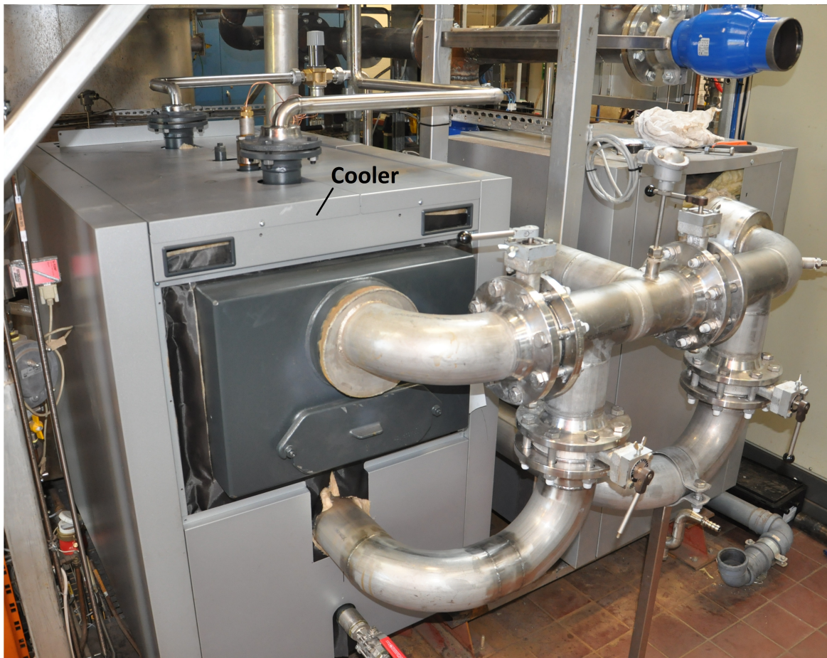
Figure A.2: Picture of the cooler located after the combustion reactor in Figure 2.1, the one used in the technical scale experiments at Chalmers 100kW oxy-fuel unit.
