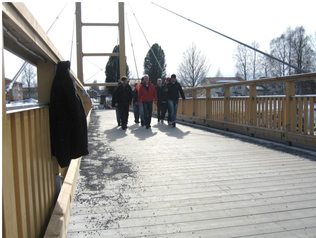
Figure 22 One of the walking tests at Älvsbackabron with controlled walking frequency.
