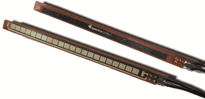
Figure 10: The SpectraSymbol Flex Sensor. Some of the most common uses for this sensor is in robotics, gaming and medical devices.
