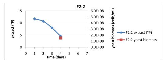
**Figure 4.2** Yeast biomass and extract during 2<sup>nd</sup> round of propagation from first yeast batch.
