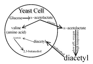
**Figure 2.9** Illustration of compounds involved during diacetyl formation and reduction inside and outside of the yeast cell (Stueven, 2003).
