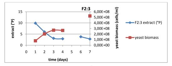
**Figure 4.3** Yeast biomass and extract during 3<sup>rd</sup> round of propagation from first yeast batch.
