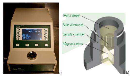
**Figure 2.5** ABER Lab Yeast Analyser (a) (Martin Marais, 2010. [Photograph]); Schematic illustration of the sample chamber of Lab Yeast Analyser (b) (Aber Intruments, 2010).
