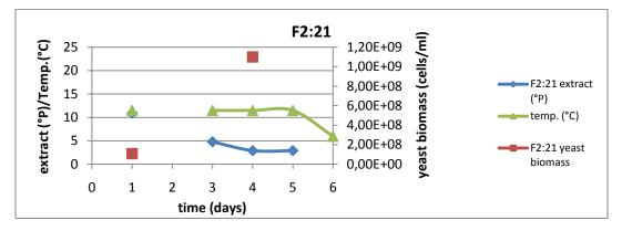
**Figure 4.5** Yeast count, extract and temperature during 1<sup>st</sup> round of propagation in second yeast batch.
