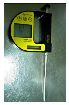
Figure 2.4 Extract measurement device called density meter (Martin Marais, 2010 [Photograph]).
