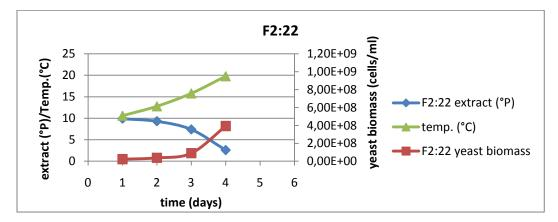
**Figure 4.6** Yeast count, extract and temperature during 2<sup>nd</sup> round of propagation in second yeast batch.
