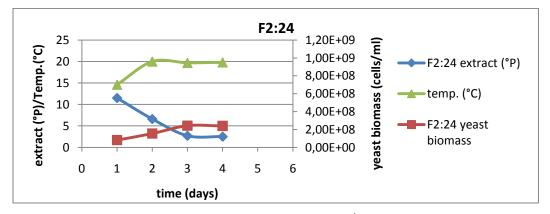
**Figure 4.8** Yeast count, extract and temperature during 4<sup>th</sup> round of propagation in second yeast batch.
