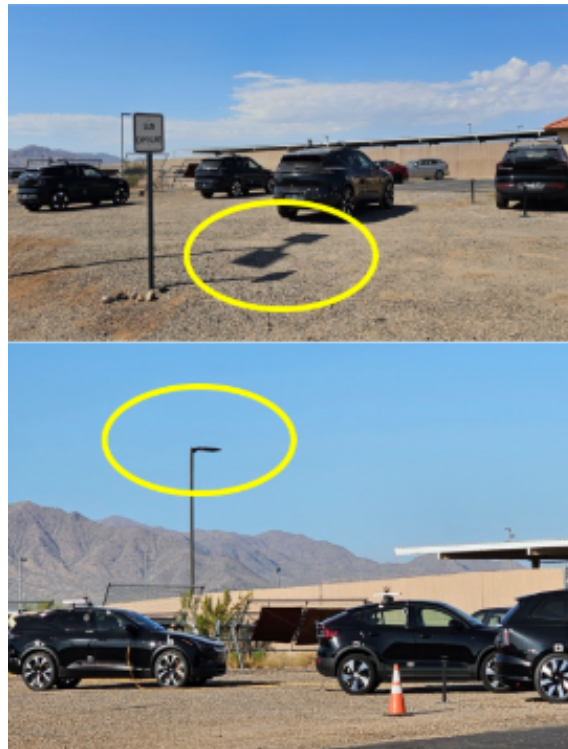
Figure 5.4: Localized dark spots caused by a floodlight at the proving ground
