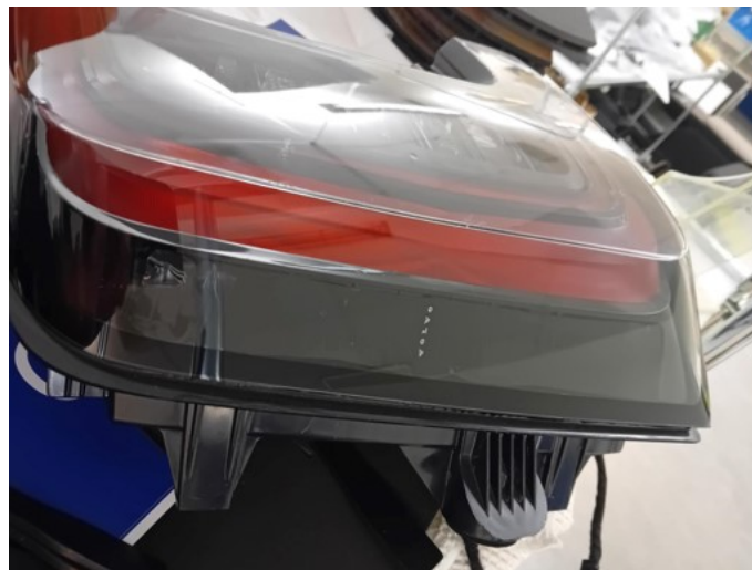
Figure 4.11: Black IR transparent reflex reflector on the left lamp
