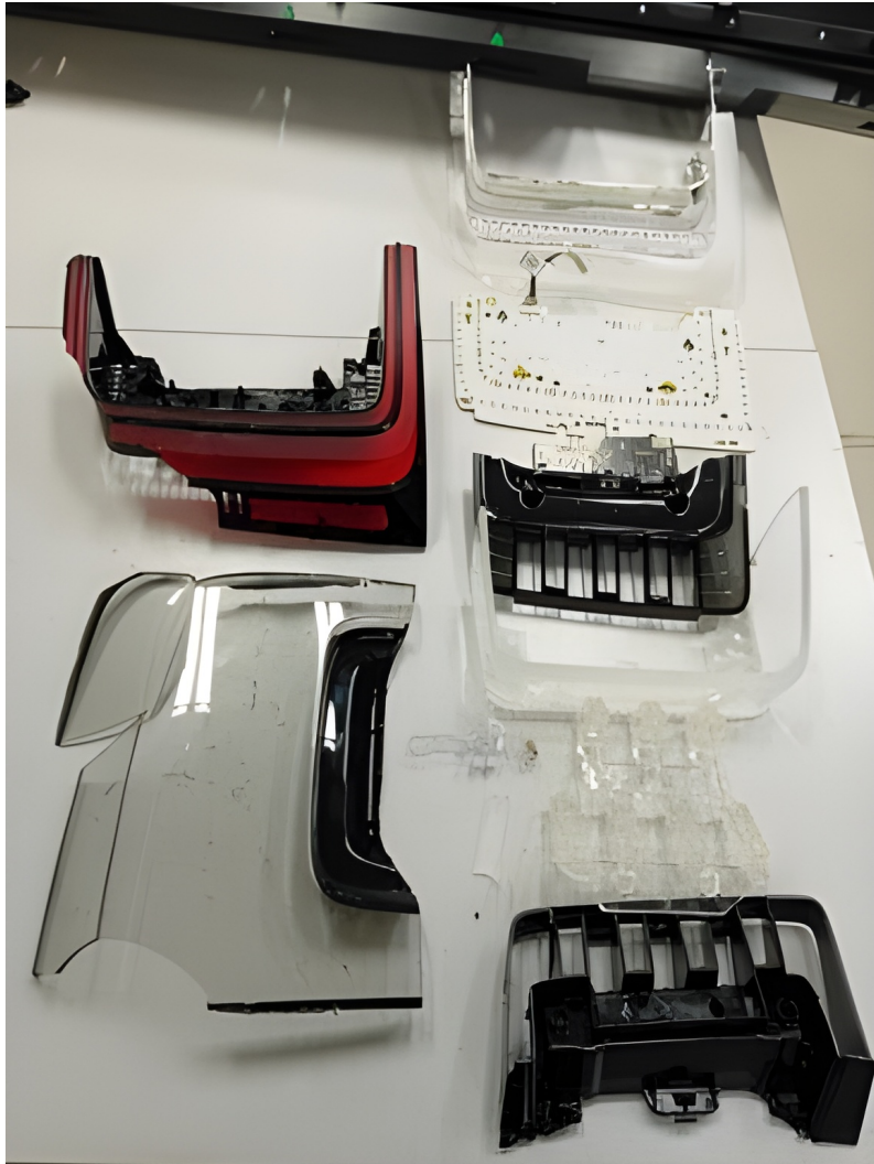
Figure A.1: Segregated rear lamp
