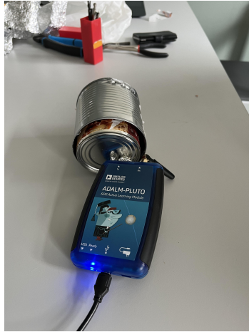
(a) Setup of leakage test with one module
