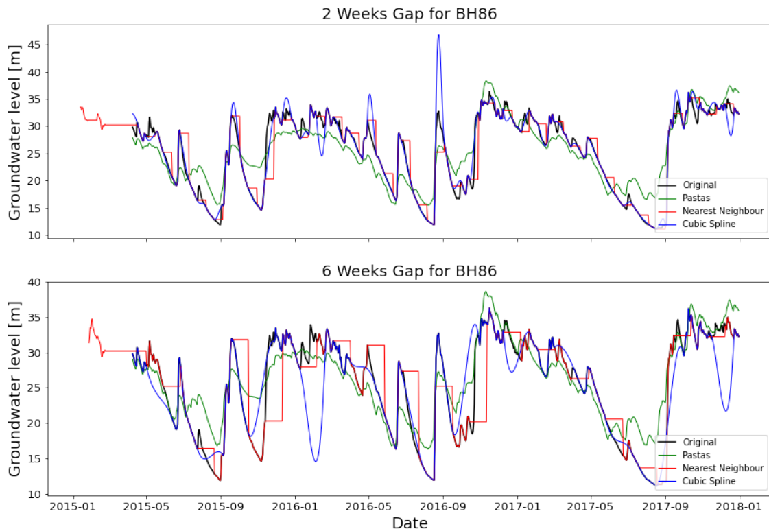
Figure 8.56: a) Every two weeks of the time-series is calibrated or simulated for b) Every six weeks of the time-series is calibrated or simulated for
