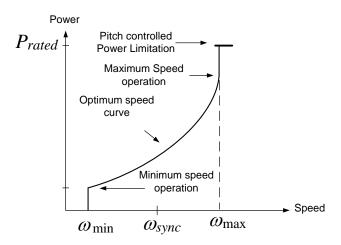
Figure 3.5: Power-speed curve
