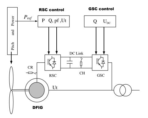
Figure 3.4: Typical layout of a DFIG
