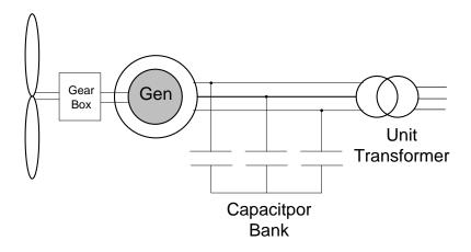
Figure 3.1: Fixed speed wind turbine
