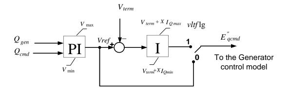
Figure 3.20: Voltage control model
