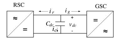
Figure 3.8: dc-link equivalent circuit
