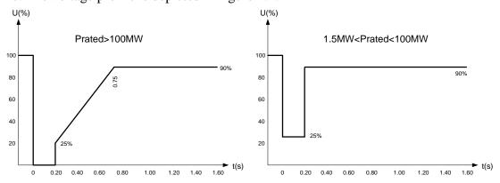
Figure 4.1: Voltage profile for wind farm to perform fault-ride through
