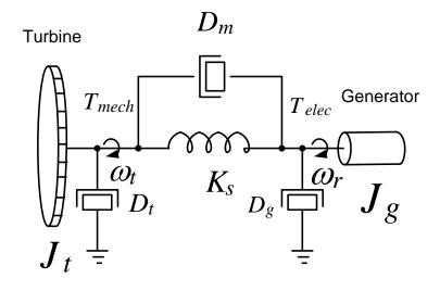
Figure 3.11: Drive Train of Wind Turbine
