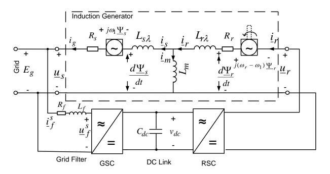
Figure 3.3: Dynamic equivalent circuit of the DFIG and converters
