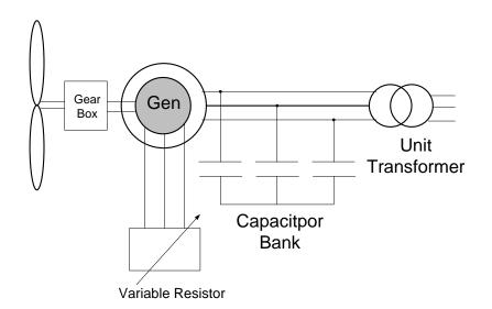
Figure 3.2: Variable-speed wind turbine with variable rotor resistance
