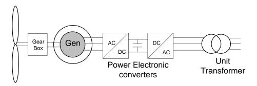
Figure 3.4: Full converter wind turbine
