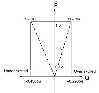
Figure 4.3: GE 1.5 MW DFIG capability curve
