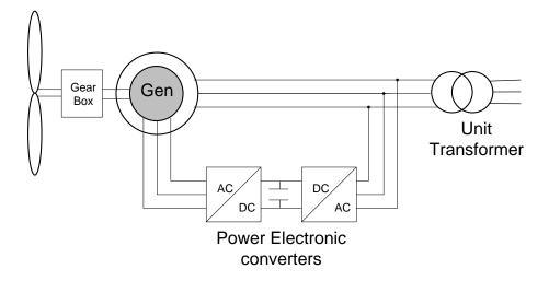
Figure 3.3: Variable-speed with doubly fed induction generator
