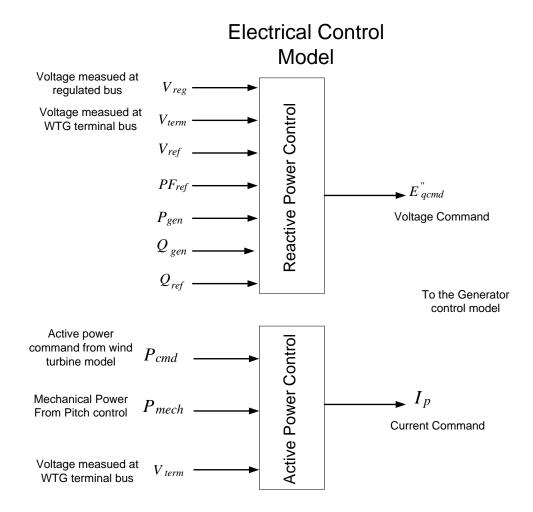
Figure 3.21 Overall DFIG electrical control model
