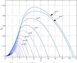
Figure 3.13: Wind power C<sub>p</sub> curves
