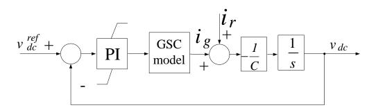
Figure 3.9: Simplified model of the dc-link and the grid-side converter.
