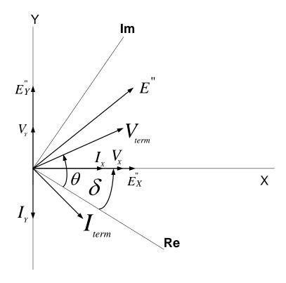
Figure 3.18: Vector diagram of voltages and currents
