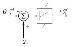
Figure 3.6: Rotor current controller: (a) active and (b) reactive power control
