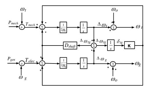
Figure 3.12: Two-mass torsional model
