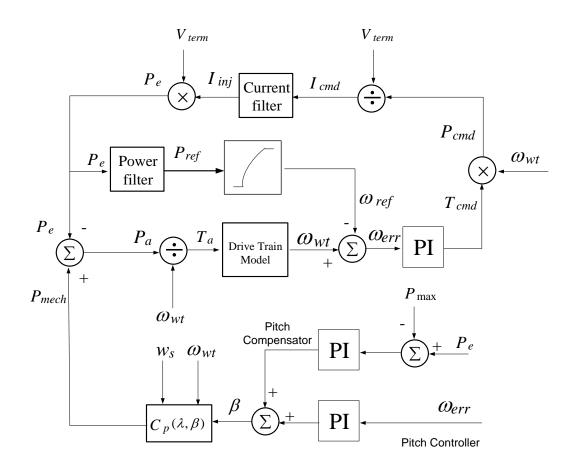
Figure 3.15: The block diagram for active power control in wind turbine
