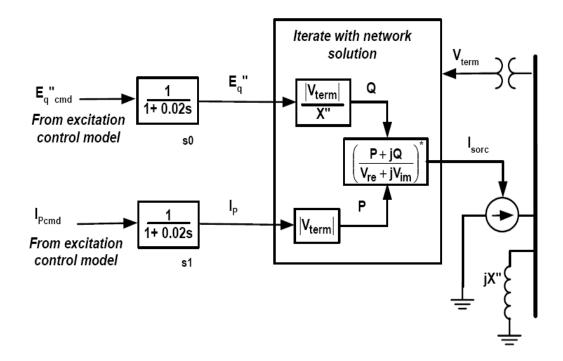
Figure 3.17: Generator and rotor converter model
