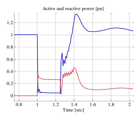
Figure 4.15: Active and reactive power profile for upper limit value of 0.55pu
