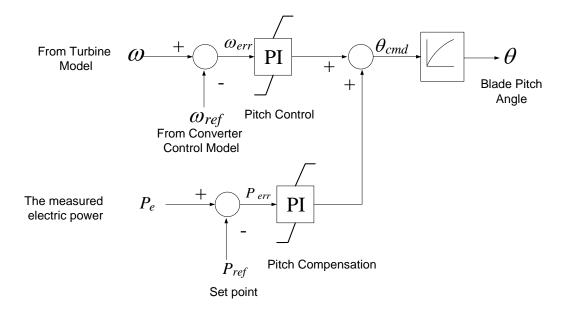
Figure 3.14: Pitch control and pitch compensation block diagram
