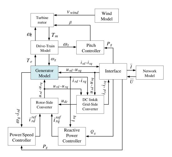
Figure 3.2: Control block diagram of DFIG wind turbine
