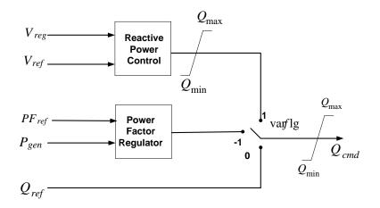
Figure 3.19: Converter control model
