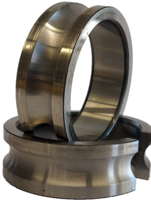
Figure 24 Picture of the ring, showing the cut made for the prepared sample
