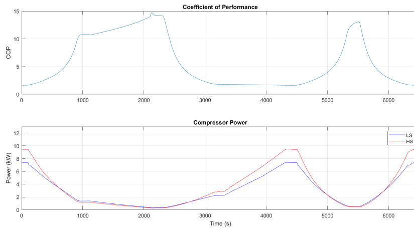
Figure 4.11: Coefficient of performance and compressor power consumption.
