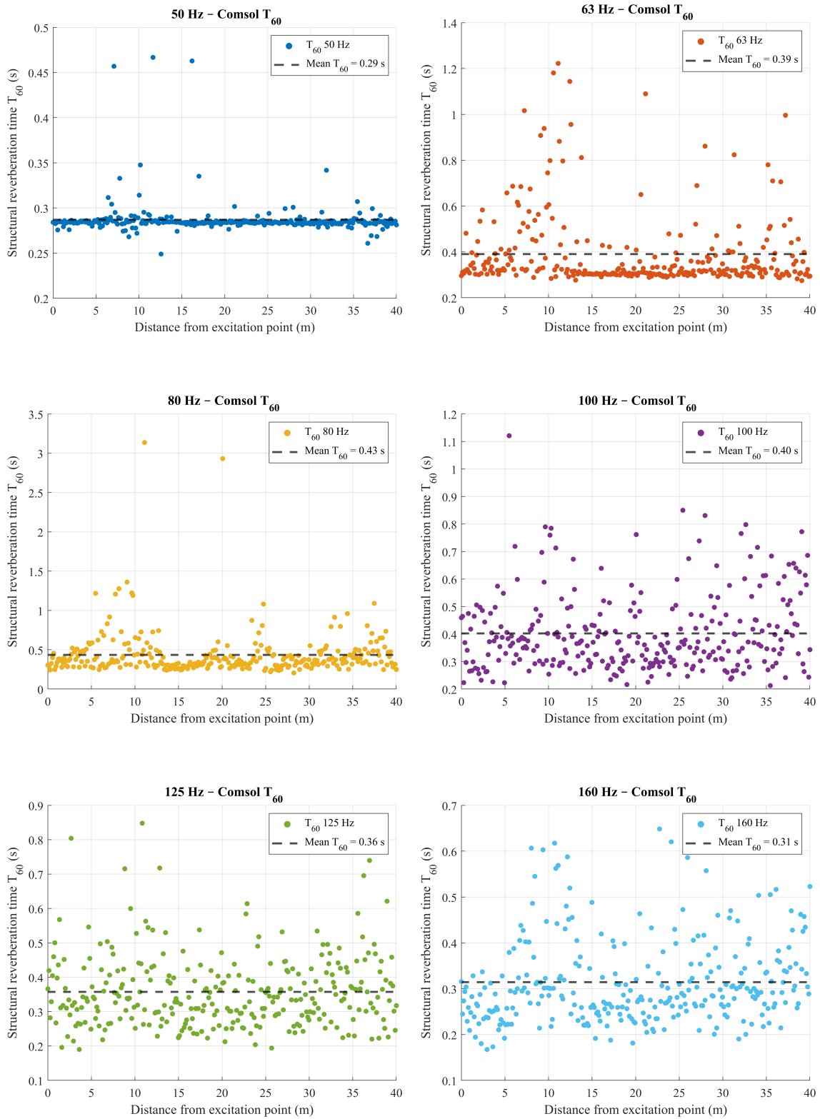
Figure 4.2: Simulated reverberation time, T_{60} , across one-third-octave bands based on Cmsol simulations.
