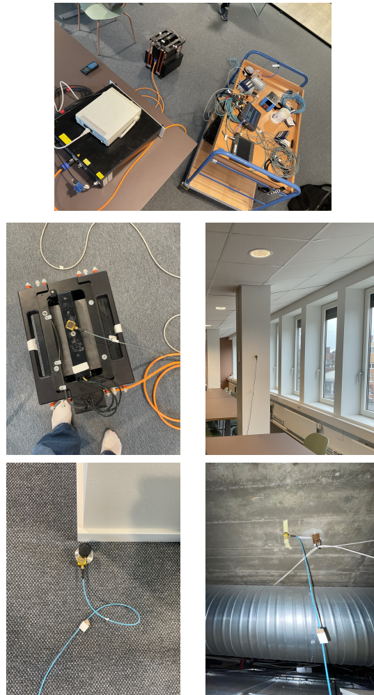
Figure 3.3: Measurement setup and accelerometer placements. Top: overview of the equipment used. Middle left: accelerometer on the shaker, middle right: on pillar (P7). Bottom left: on the floor slab (M1). Bottom right: on the roof structure (M23).
