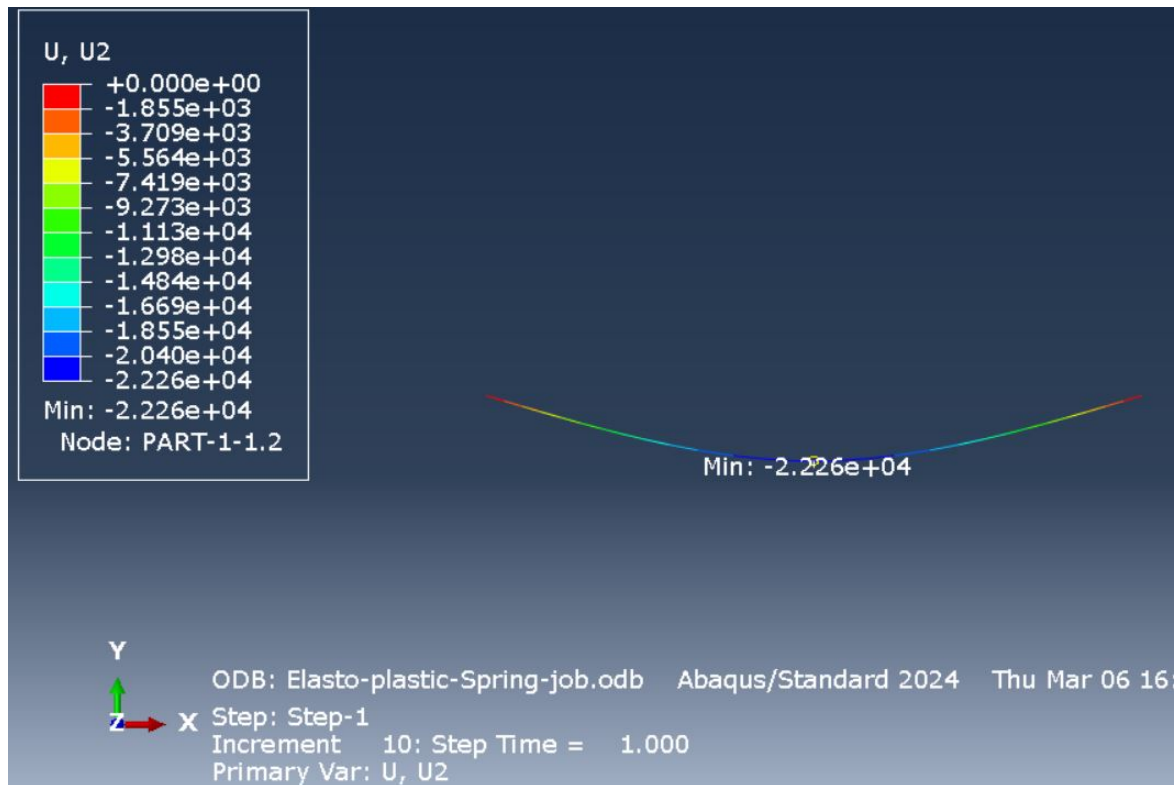
Figure E.6: Displacement with NL-springs at 10 kN
