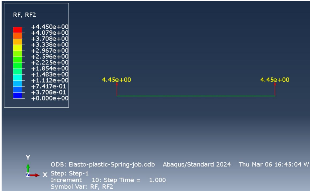
Figure E.7: Support reactions with NL-springs at 10 kN
