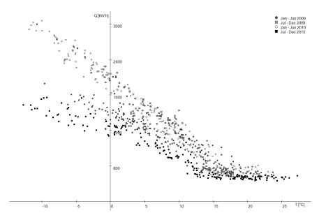
Figure 7: T-Q plot for building 1961 with different colors for different periods.
