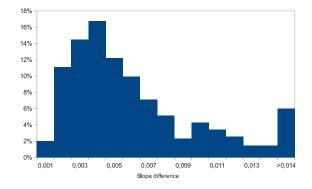
Figure 11: Distribution of the slope difference parameter for the buildings in the dataset. The median value is 0,0044.
