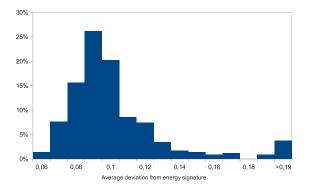
Figure 9: Distribution of the average deviation from the energy signature. A low value means that the data closely matches the energy signature. The mean value is 0,10 while the median is 0,089.
