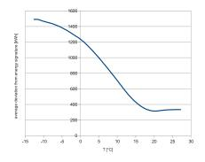
Figure 6: The average deviation from the fitted spline for building 1574. The spline consists of two segments, the segment at the right has zero slope.
