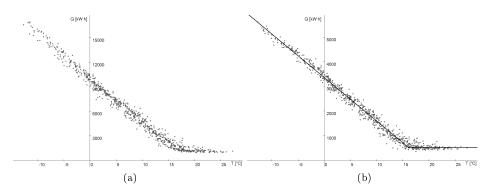
Figure 3: The left figure shows a plot where the daily energy for building 869 is plotted against the outside temperature. The figure on the right shows a similar plot for building 1973 and also shows the energy signature for the building marked with two black line segments.
