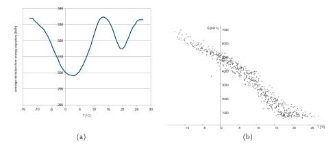
Figure 5: The figure on the left shows the average deviation from the fitted spline plotted against the position of the knot for building 1574. The figure on the right shows the T-Q plot for this building.
