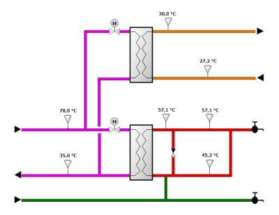
Figure 1: A typical control system for heating and hot water for the studied buildings. The upper two lines on the left are connected to the district heating. The supplied energy is used both for heating the building and for the hot water used by the tenants. The upper two lines on the right side are connected to the radiators. The lowest tap represents cold water used by tenants, while the upper tap represents hot water.
