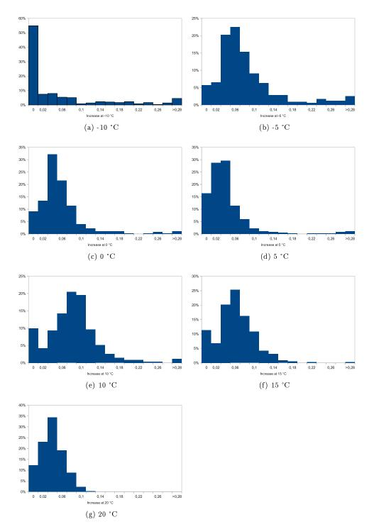
Figure 13: Distributions of the increase in the energy signature at different temperatures.
