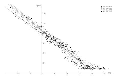
Figure 12: The T-Q plot for building 1058, different colors are used for the different periods. The slopes for the data from the different periods is marked with black lines. From top to bottom: Jan-Jun 2010, Jul-Dec 2010, Jul-Dec 2009 and Jan-Jun 2009.
