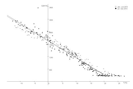
Figure 8: The energy signature for building 2477 has very little difference between the slopes for the different periods plotted. The difference between these periods is substantial nonetheless. The lower slope belongs to the first half of 2010, the upper to the second half.
