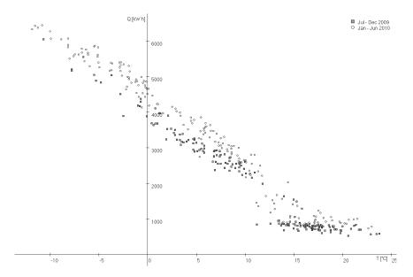
Figure 10: The T-Q plot of building 585, the building with the median value of deviation from the energy signature in the total set of buildings. Large differences between the two plotted periods exist in the amount of energy used at temperatures below 10 °C.
