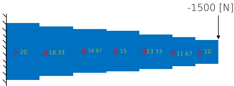
Figure 4.3: Stepped cantilever beam element.
