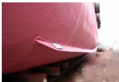
Figure 1.2: "Bilge keel on a steel vessel" by Dj245 at en.wikipedia is licensed under CC BY-SA 3.0 [5]
