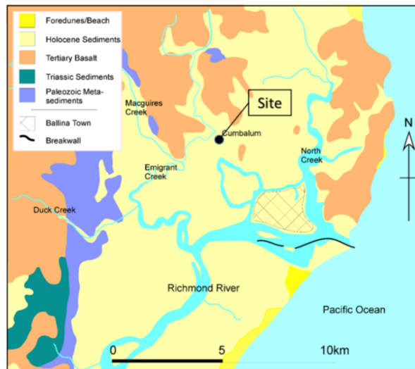
Figure 3.2. Geological setting of the Ballina National Field-Testing Facility (NFT) (Pineda, et al., 2019).
