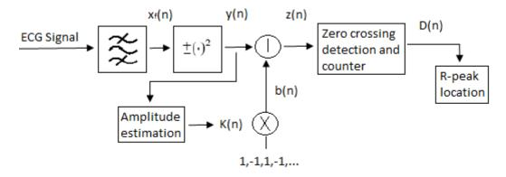
Figure 2.8: Block diagram for algorithm 1
