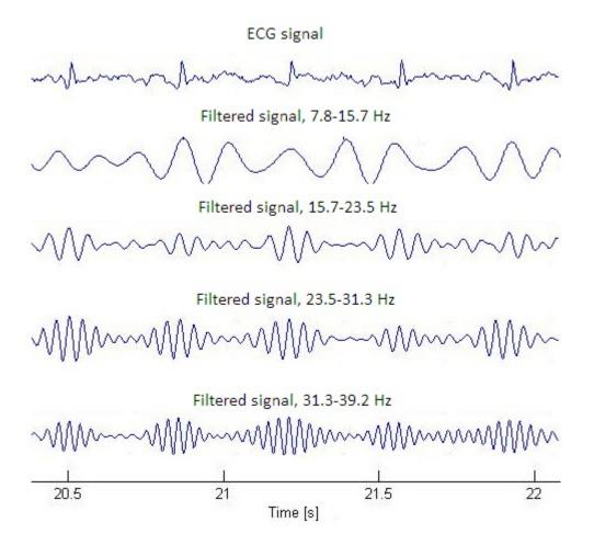
Figure 2.13: Preprocessing steps for algorithm 3
