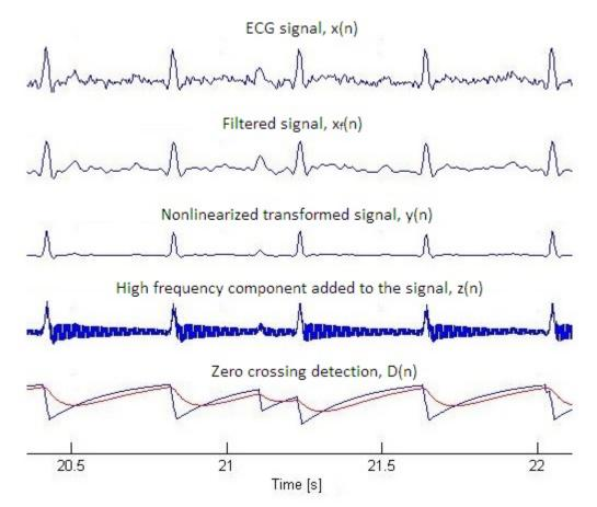
Figure 2.9: Preprocessing steps for algorithm 1
