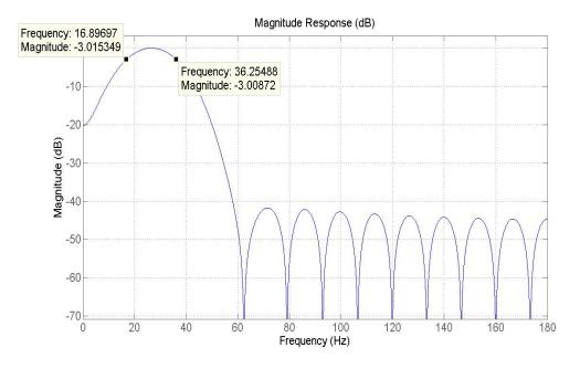
Figure 2.1: Frequency response and the cut-off frequencies for the adult ECG signal
