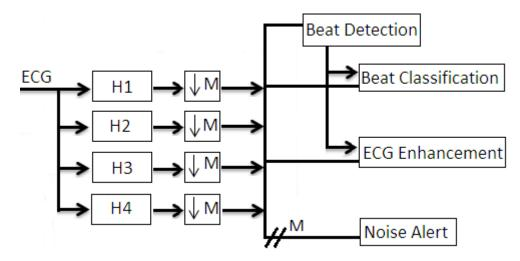
Figure 2.12: Block diagram of algorithm 3
