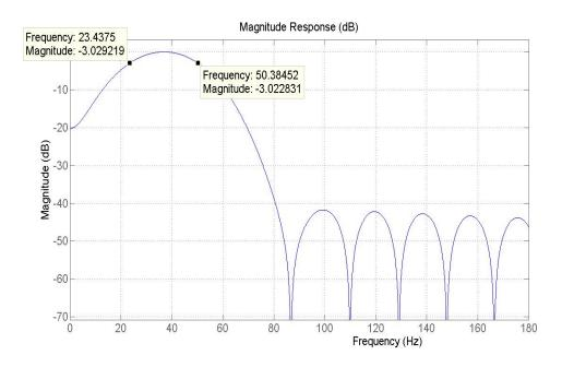
Figure 2.2: Frequency response and the cut-off frequencies for the fetal ECG signal
