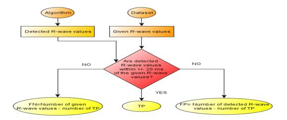
Figure 2.3: Flow chart of the validation for the adult ECG signal
