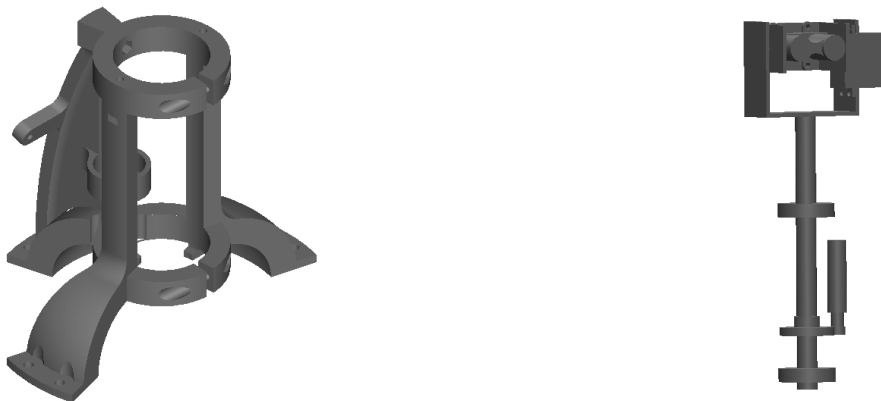
Figure 4.1: Left: CAD model of the 3D-printed scanner platform. Right: Principal layout of the rotational components.
