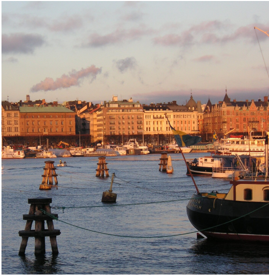
Figure 1.1: Old mooring dolphin featuring timber piles. Comment: Adapted from: Vy från Skeppsholmen mot Strandvägen i Stockholm [photo], of H. Ellgaard, 2005, Wikimedia Commons. Licensed under CC-BY-SA-3.0.
