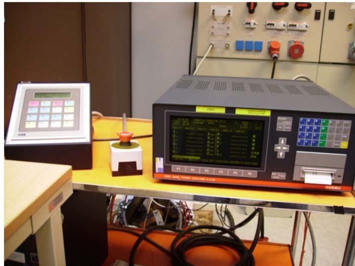
*Figure 4.5 The power analyser (right) and generator control (left).*
