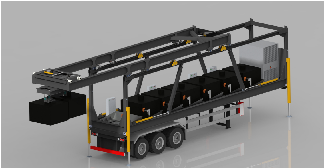
Figure 4.19: Rendering of final CAD model of the BSMS.
