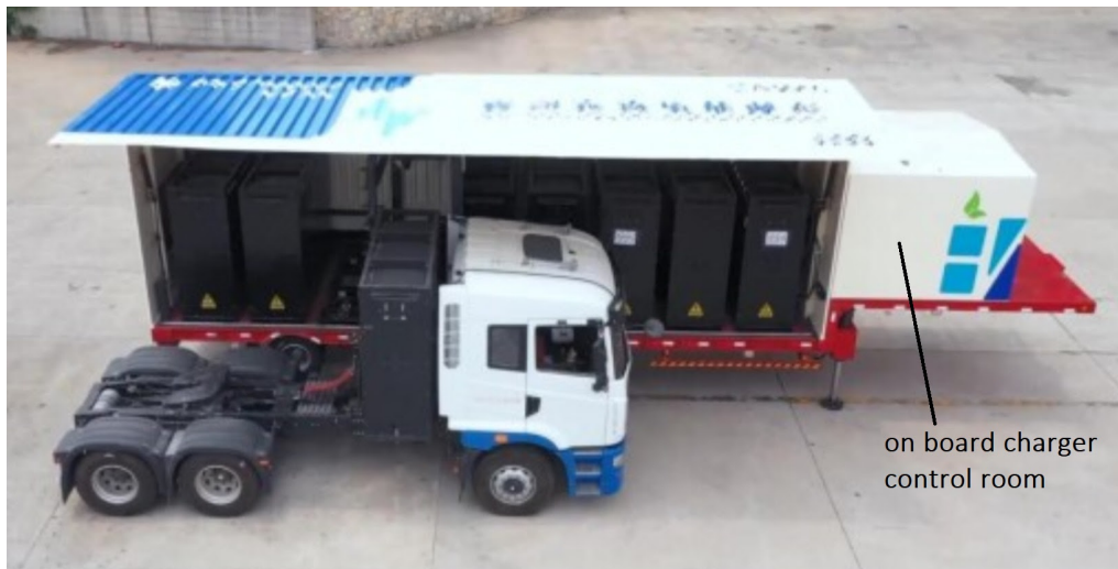
Figure 4.2: XCMG Battery Swap Solution [31].
