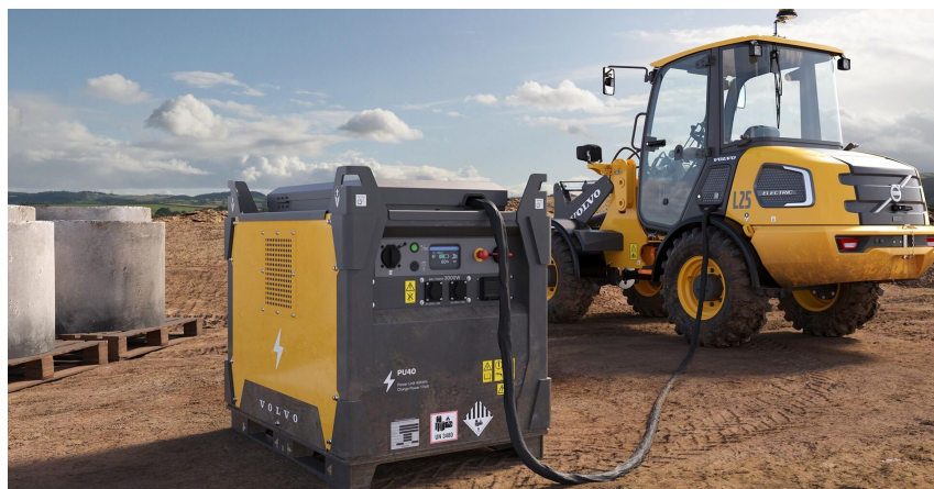
Figure 1.1: Volvo L25 Wheel Loader being charged by an external BPU [6].
