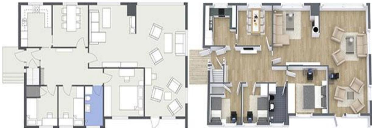
**Figure 9 - 2D floor plan compared with 3D floor plan (Roomsketcher, 2016)**
