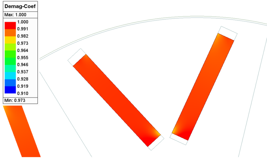
Figure 4.22: Demagnetization coefficient distribution of the NdFeB VPMSM after the three-phase short-circuit demagnetization study at -40^{\circ}\text{C} .
