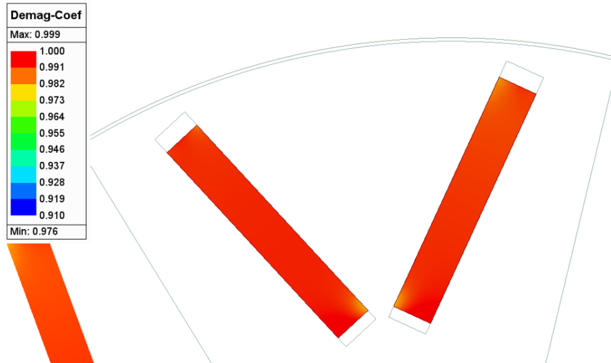
Figure 4.23: Demagnetization coefficient distribution of the NdFeB VPMSM after the three-phase short-circuit demagnetization study at 20^{\circ}\text{C} .
