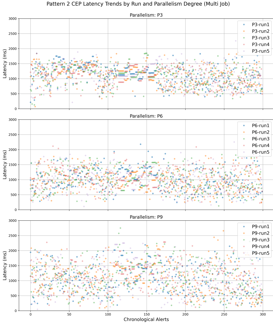
Figure 5.24: Pattern 2: Multi-job SP query latency trend as a function of run number and degree of parallelism for the CEP query. The plot displays a representative sample of 300 data points.
