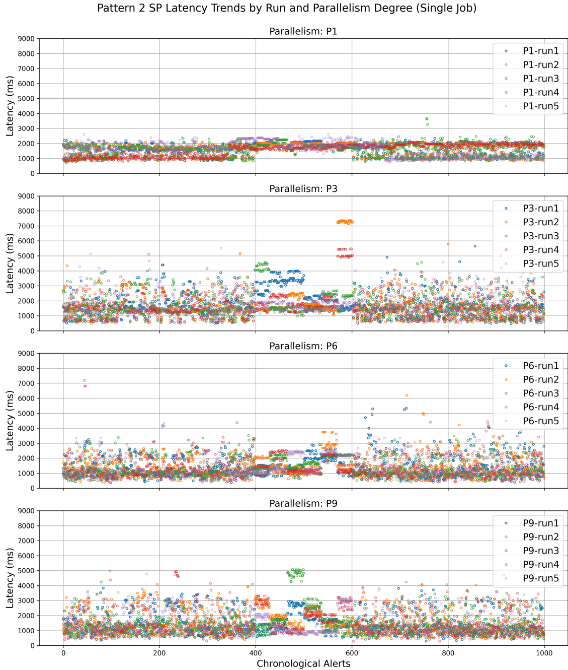
Figure 5.17: Pattern 2: Single-job SP query latency trend as a function of run number and degree of parallelism for the SP query of Pattern 2. The plot displays a representative sample of 1000 data points.
