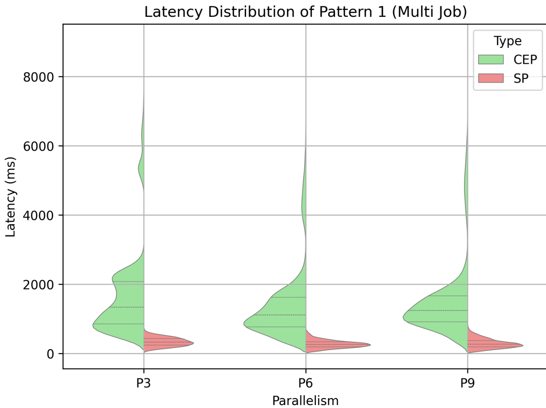
Figure 5.10: Pattern 1: Multi-job latency distribution across parallelism levels for CEP and SP query.
