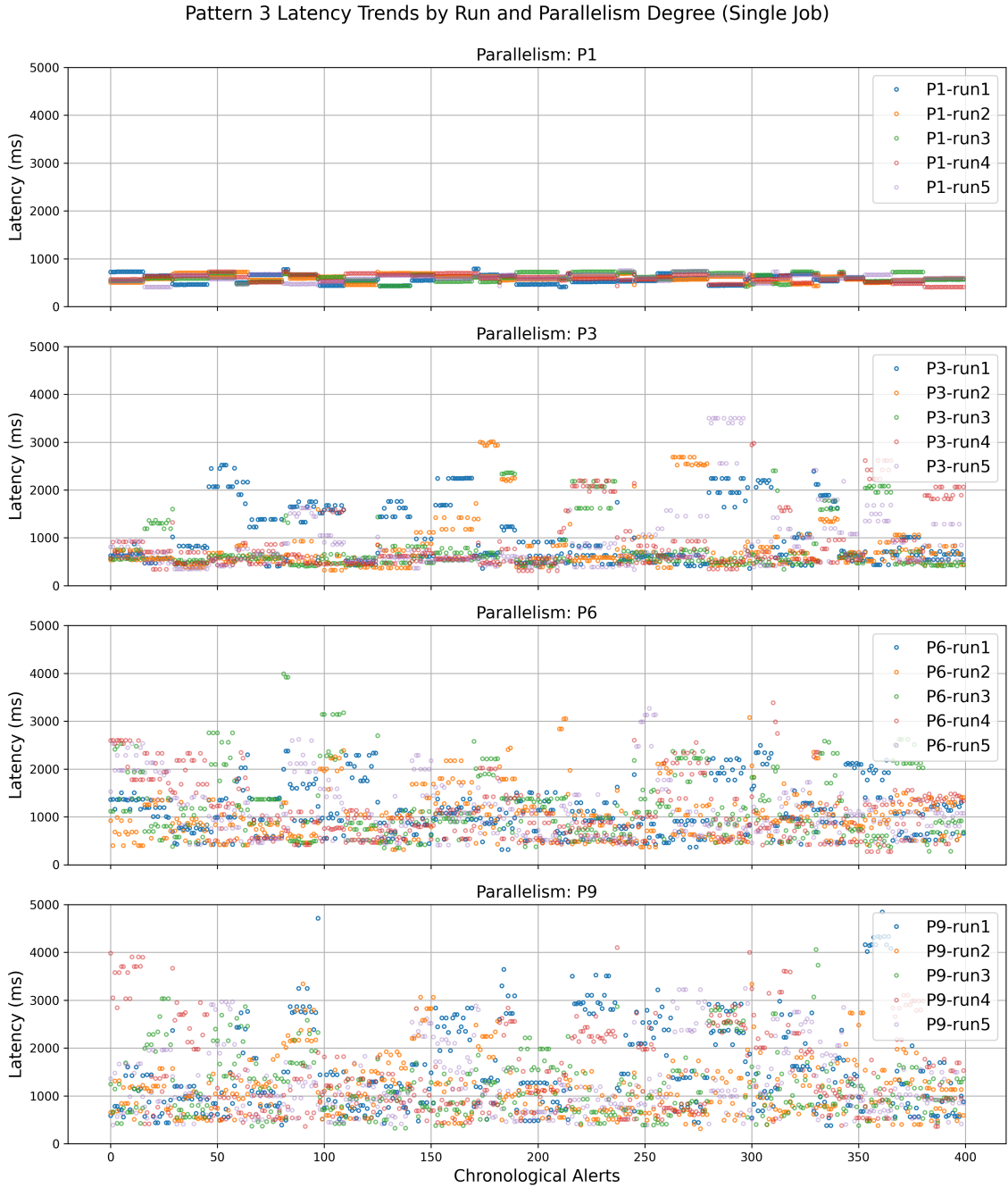
Figure 5.29: Pattern 3: Single-job latency as a function of run number and degree of parallelism. The plot displays a representative sample of 400 data points.
