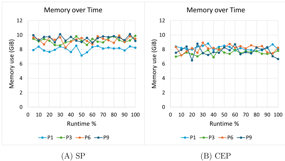
Figure 5.3: Pattern 1: Single-job memory usage over time for varying levels of source parallelism. Each point on the x-axis represents the average memory usage over a consecutive 5% segment of the job's total runtime. (A) shows the SP query; (B) shows the CEP query.
