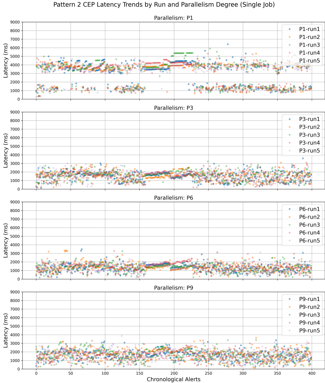
Figure 5.18: Pattern 2: Single-job SP query latency trend as a function of run number and degree of parallelism for the CEP query. The plot displays a representative sample of 400 data points.
